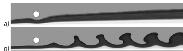
Fig. 9. Temperature Contour Plots for a) Re = 2000 , \beta = 0.2 b) Re = 2000 , \beta = 0.3
