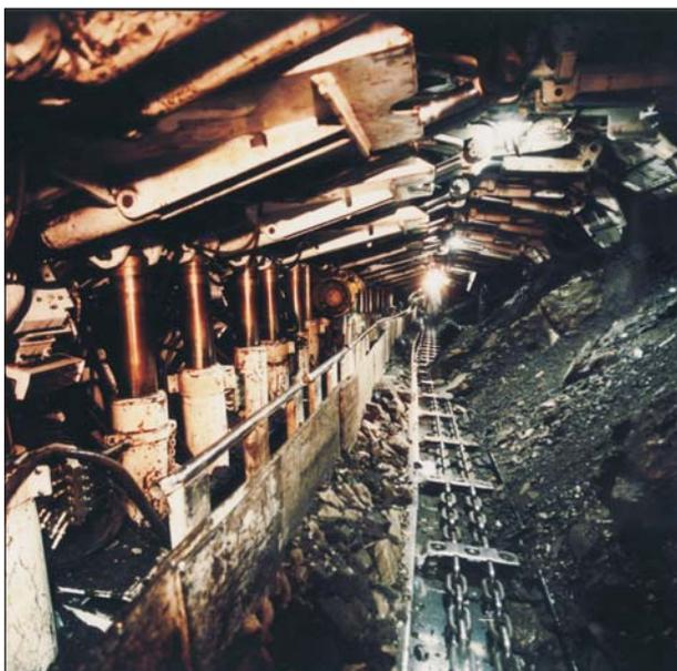
Figure 2. Longwall operation in the Velenje coal mine.
