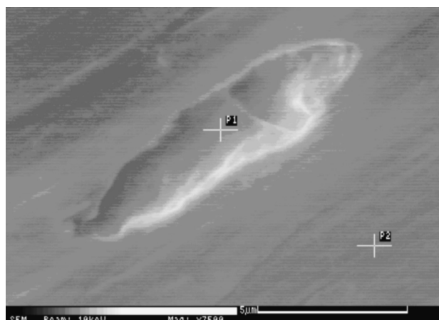
Figure 9: Surface with corrosion pit. At the points P1 and P2 the AES analyses were performed. The presence of Cl was detected only in the pit. SEM
