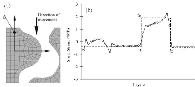
**Figure 2:** Shear stresses at point A within a complete loading cycle
