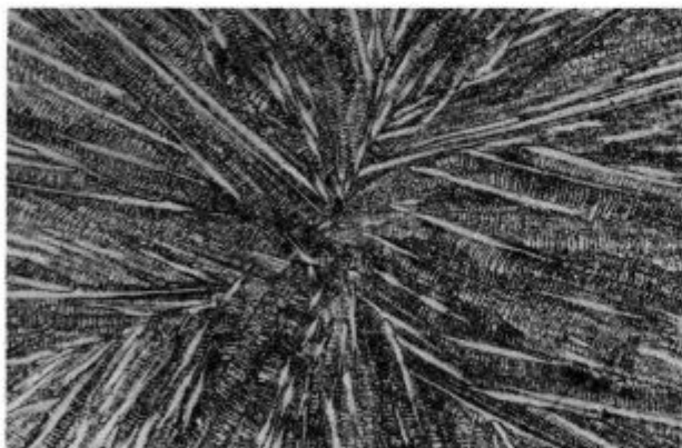
Slika 3: Mikroposnetek konti lite žice po litju (pov. 50 ×) Fig. 3: Microstructure of continuously cast steel (magn. 50 ×)
