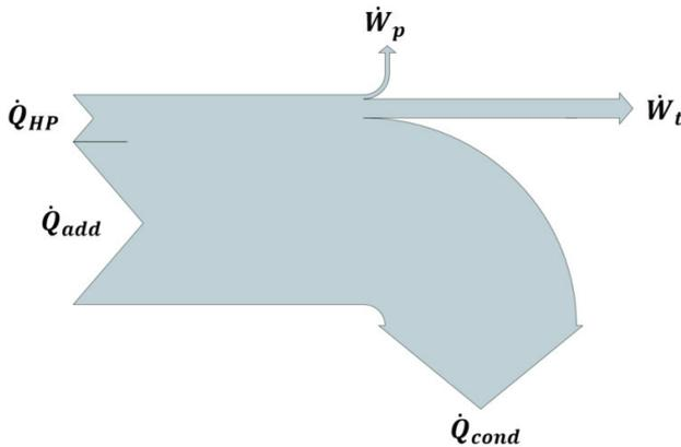
**Figure 4:** ORC system power flow diagram
