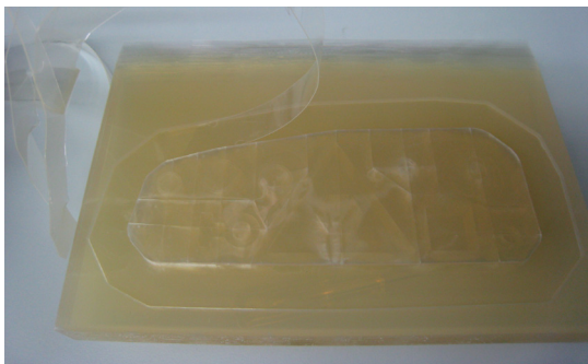
Fig. 11. Waste-material removal in LOM
