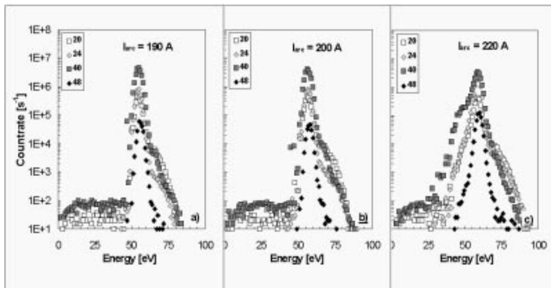
**Figure 5:** Energy spectra of Ti ( $m/q=24, 48$ ) and Ar ( $m/q=20, 40$ ) single and double charged ions during TiN deposition for different arc currents; other conditions are standard one (Table 1): a)  $I_{\text{arc}}=190$  A, b)  $I_{\text{arc}}=200$  A, standard conditions, c)  $I_{\text{arc}}=220$  A
