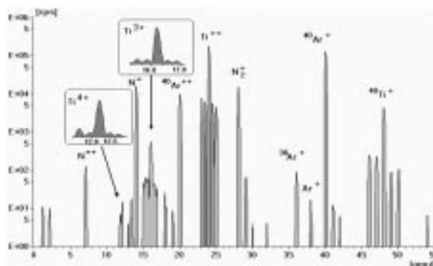
**Figure 3:** Mass spectrum during standard TiN deposition measured at the peak energy 55 eV. The inserts show the fine structure of the peaks corresponding to  $\text{Ti}^{3+}$  ( $m/q=16$ ) and  $\text{Ti}^{4+}$  ( $m/q=12$ ) ions
