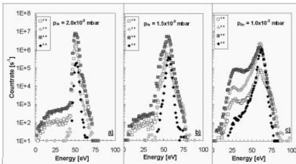
**Figure 4:** Energy spectra of Ti ( $m/q=24, 48$ ) and Ar ( $m/q=20, 40$ ) single and double charged ions during TiN deposition for different Ar pressures; other conditions are standard one (**Table 1**): a)  $p_{\text{Ar}}=1.0 \times 10^{-3}$  mbar, b)  $p_{\text{Ar}}=1.5 \times 10^{-3}$  mbar, standard conditions, c)  $p_{\text{Ar}}=2.0 \times 10^{-3}$  mbar
