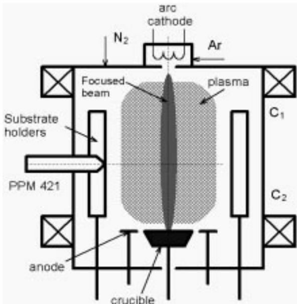
**Figure 1:** Scheme of the triode ion plating system Balzers BAI 730 M
