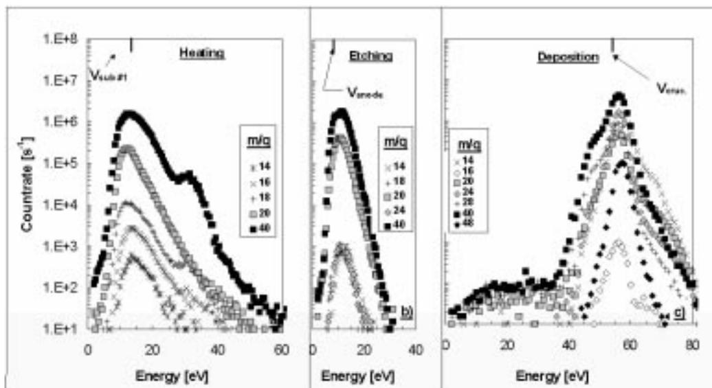
**Figure 2:** Energy spectra of various positive ions for standard heating: (a), etching (b) and TiN deposition process (c)
