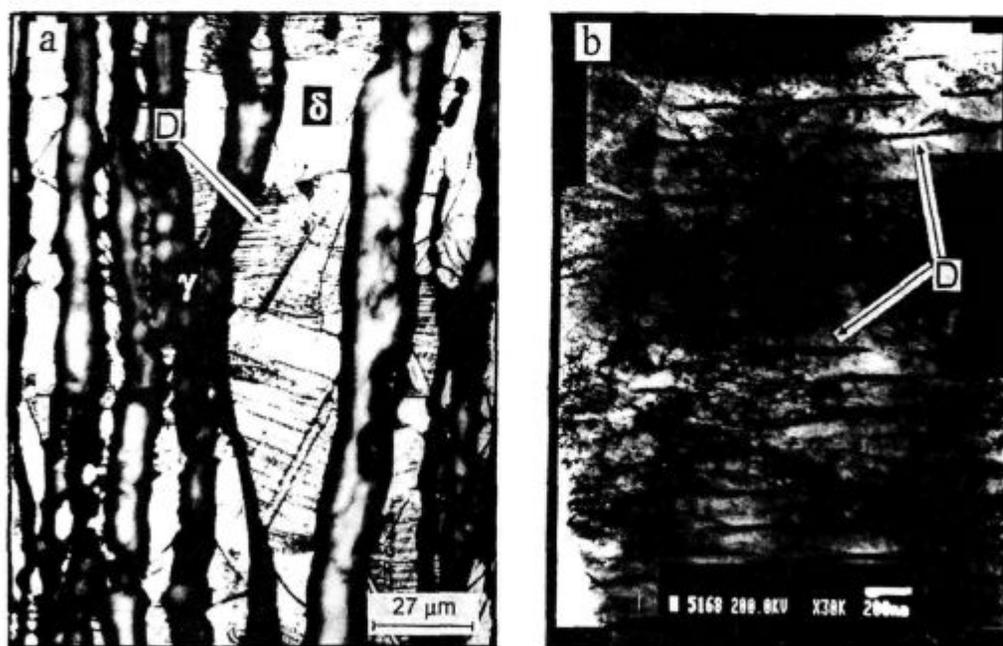
Figure 4: Optical (a) and transmission electron bright-field micrographs (b) of duplex steel. D - twins
