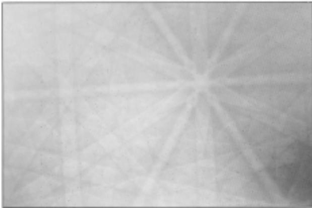
**Figure 15:** Electron back-scattered pattern (Kikuchi pattern) obtained by interaction of the primary electron-microscope beam with austenite specimen<sup>17</sup>
