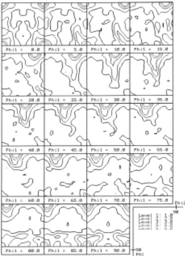
**Figure 11:** ODF sections at constant angle  $\phi_1$  determined on the surface of electrical steel alloyed with 0.05 %Sn
