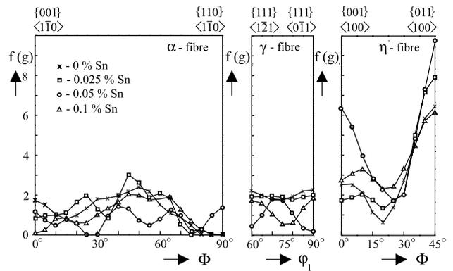
**Figure 13:** Quantitative description of  $\alpha$ ,  $\gamma$  and  $\eta$  fibre intensity which allows the direct comparison of a certain orientation density, in this case four electrical steels alloyed with different Sn content
