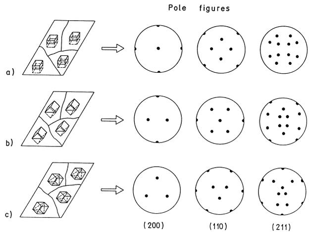
**Figure 5:** Schematic {200}, {110} and {211} pole figures for steel sheet with idealised textures (a) {100}<001>, (b) {110}<001> in (c) {111}<112>
