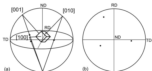
**Figure 2:** (a) Family of  $\{001\}$  poles in a cubic crystal projected onto the reference sphere of a stereographic projection (b) Pole figure of one crystal
