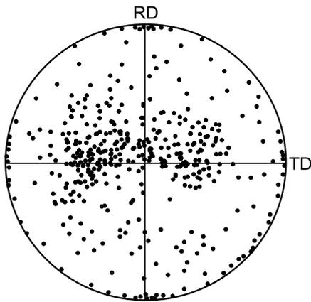
**Figure 3:** {001} pole figure of electrical steel alloyed with 0.05 %Sb
