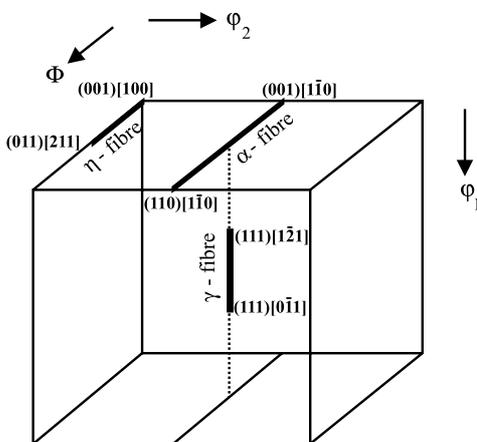
**Figure 12:** Euler space with marked  $\alpha$ ,  $\gamma$  and  $\eta$  fibres
