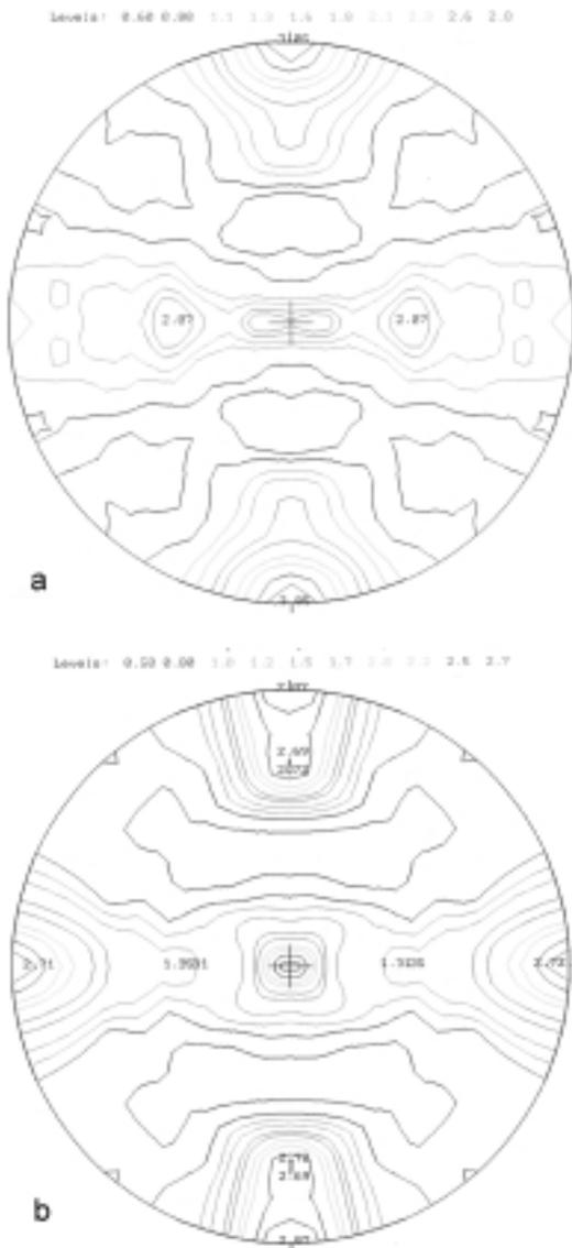
**Figure 4:** {200} computed pole figures measured on the surface of electrical steel (a) without Sn and (b) with 0.05 %Sn
