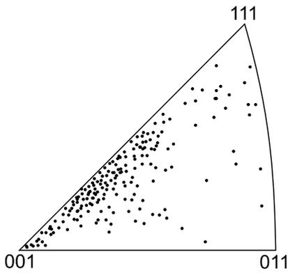
**Figure 7:** Inverse pole figure of the electrical steel alloyed with 0.05 %Sb
