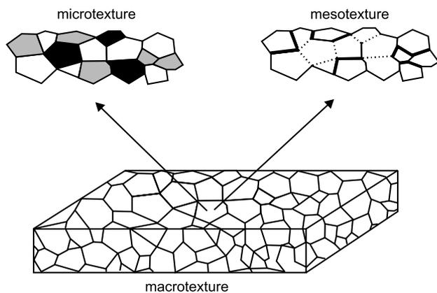
**Figure 1:** Schematic diagram illustrating the relationship between macrotexture, microtexture and mesotexture. The macrotexture represents the grain orientation of the sample, the microtexture represents the grain orientation of a smaller area, in this case fifteen grains with three different orientation categories and the mesotexture where, for example, three boundary types are indicated
