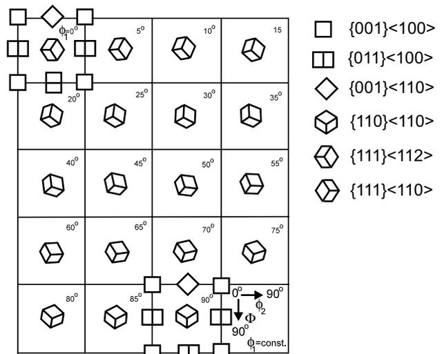
**Figure 10:** ODF sections showing the location of some orientations
