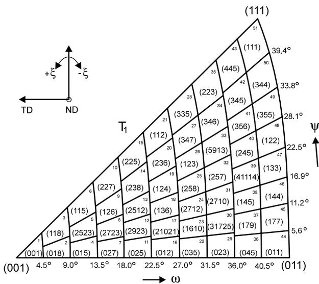
**Figure 8:** The areas of determined orientations in the unit stereographic triangle
