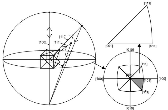
**Figure 6:** The inverse pole-figure plots direction in the sample related to fixed crystal directions in a single unit triangle of the stereographic projection
