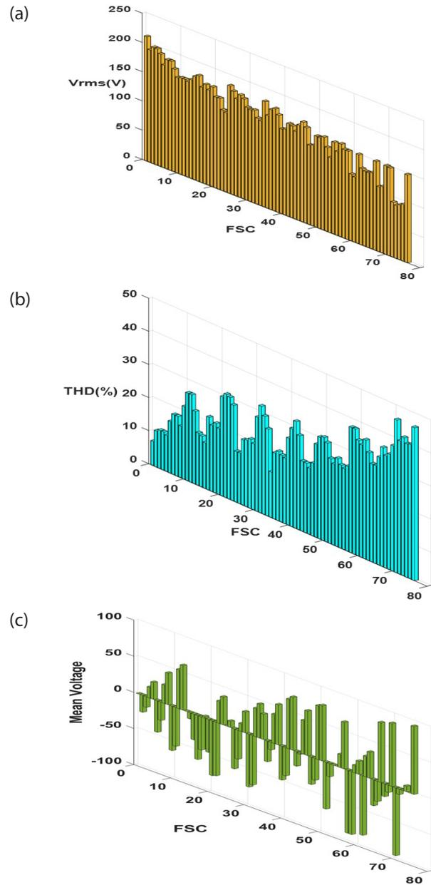
**Figure 5:** RMS voltage and THD for various Fault switch condition (FSC): (a) RMS voltage (b) THD (%) (c) mean voltage.
