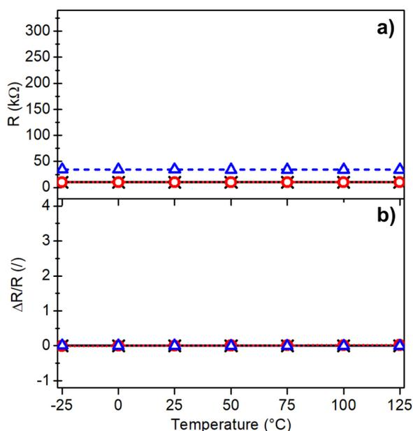
**Figure 7:** Resistances (a) and relative resistances (b) as a function of temperature for 2041-10/air ( $\times$ ), 2041-30/air ( $\circ$ ), 2041-30/Ar ( $\triangle$ ).
