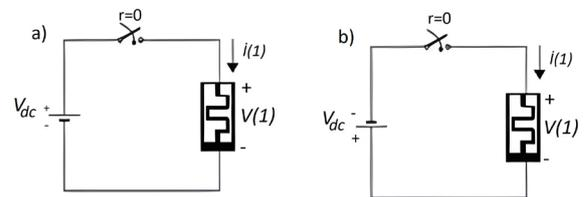
**Figure 1:** The memristor supplied by a) a positive DC voltage source for the forward resistive switching (x goes up from 0 to 1) and b) a negative DC voltage source for the reverse resistive switching (x goes down from 1 to 0)
