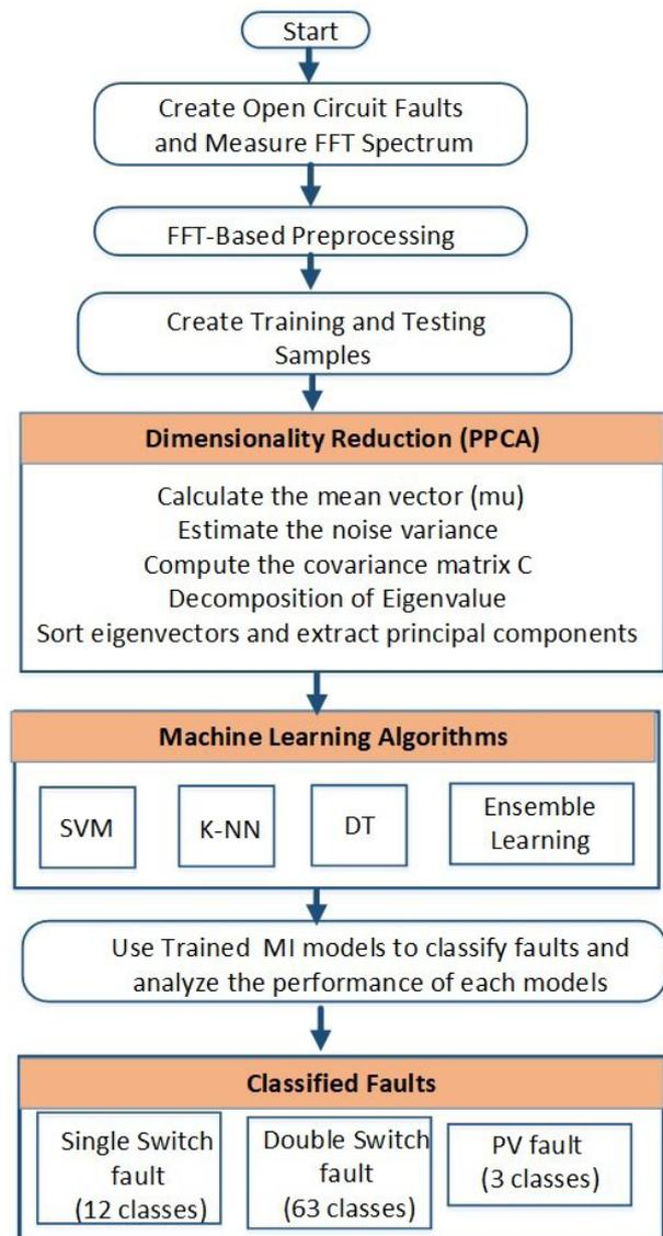
**Figure 2:** Flow chart of fault diagnosis system
