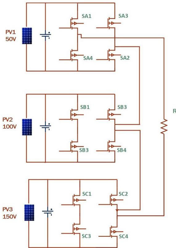
Figure 3: Circuit diagram of ACMLI
