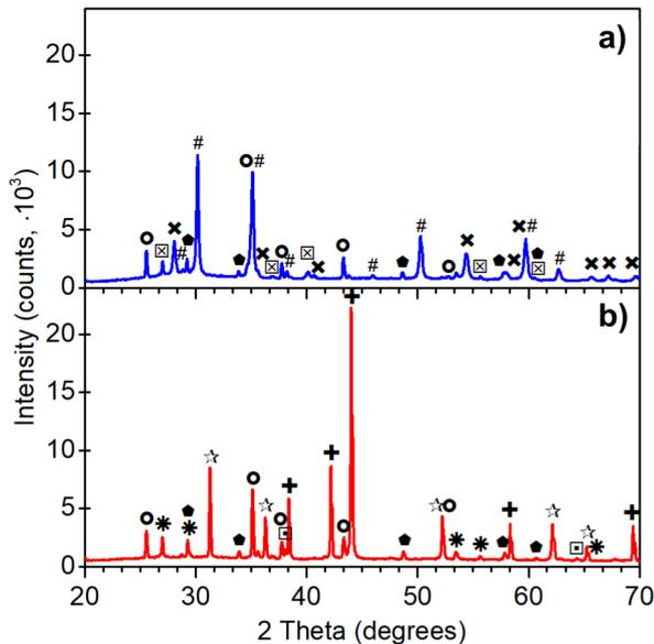
**Figure 4:** XRD patterns of a) 2041-30/air, and b) 2041-30/Ar. #:  $\text{Bi}_2\text{Ru}_2\text{O}_7$ , \*:  $\text{Bi}_2\text{O}_3$ , x:  $\text{RuO}_2$ , +: Ru, o:  $\text{PbO}_2$ , ☆:  $\text{Pb}_2\text{O}$ , ○:  $\text{Al}_2\text{O}_3$ , □: cubic  $\text{SiO}_2$  and ▣: hexagonal  $\text{SiO}_2$ .
