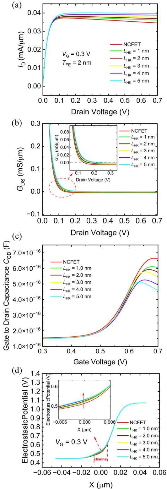
**Figure 5:** (a) Output characteristic curves as a function of the drain voltage at different  $L_{HK}$  values. (b) Output conductance curves as a function of the drain voltage at different  $L_{HK}$  values. (c) gate-drain capacitance ( $C_{GD}$ ) curves as a function of the gate voltage at different  $L_{HK}$  values. (d) Electrostatic potentials of different  $L_{HK}$  at  $V_{GS} = 0.3$  V.
