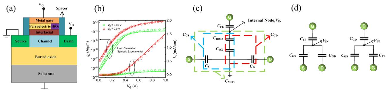
**Figure 1:** (a) Structure of the hetero-gate dielectric negative-capacitance field-effect transistor device. (b)  $I_{DS} - V_{GS}$  calibration plot of 14 nm FDSOI comparisons between technology computer-aided design (TCAD) simulation results (solid line) and experimental data (circles) [18]. (c) Equivalent capacitance circuit for negative-capacitance field-effect transistor. (d) Gate and drain control circuits.
