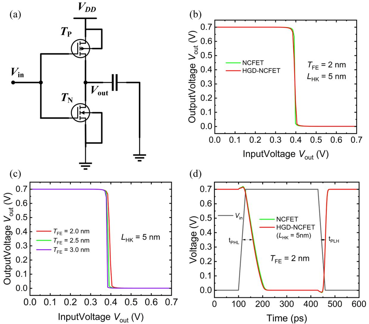
**Figure 8:** (a) implementation of CMOS inverter employing HGD-NCFET. (b) voltage transfer characteristic curves of inverter composed of NCFET and HGD-NCFET. (c) voltage transfer characteristic curves of inverter composed of HGD-NCFET at different  $T_{FE}$  values. (d) input-output waveform of inverter composed of NCFET and HGD-NCFET.
