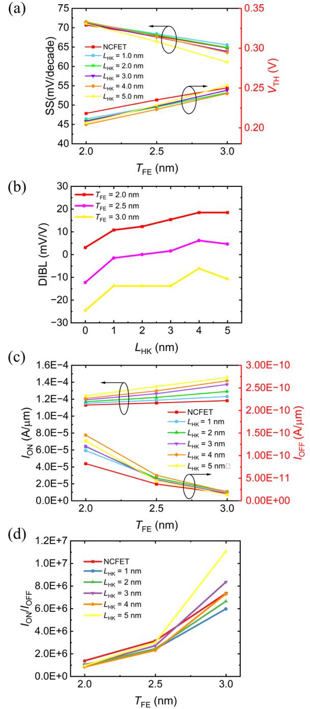
**Figure 6:** (a) Subthreshold swing (SS) and  $V_{TH}$  of HGD-NCFET at different  $L_{HK}$  settings. (b) Drain-induced barrier lowering (DIBL) effect of HGD-NCFET at different  $T_{FE}$  settings. (c)  $I_{ON}$  and  $I_{OFF}$  responses of HGD-NCFET at different  $L_{HK}$  settings. (d)  $I_{ON}/I_{OFF}$  responses of HGD-NCFET at different  $L_{HK}$  settings.
