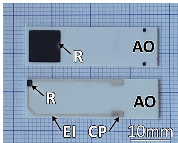
**Figure 1:** The photo of the test samples with dimensions 8.0 mm  $\times$  8.0 mm (above) and 1.1 mm  $\times$  1.1 mm (below), where R stands for resistor, EI for electrical interconnection, CP for contact pad, and AO for alumina substrate.
