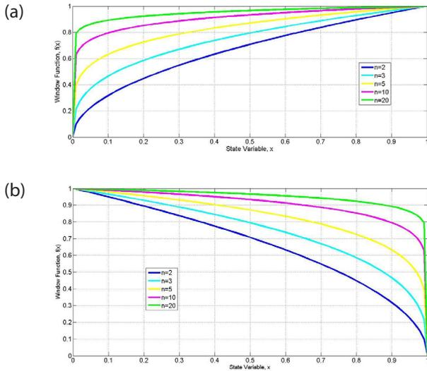
**Figure 2:** The Mutlu-Kumru window function for a) the reverse biased memristor ( $i(t) < 0$ ), various  $n$  values, and  $m_2 = 1$ , and b) for the forward biased memristor ( $i(t) > 0$ ), various  $n$  values, and  $m_1 = 1$ .
