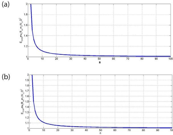
**Figure 3:** The normalized resistive switching energy of the Mutlu-Kumru memristor model with respect to the parameter  $n$  for a) the reverse biased memristor ( $i(t) < 0$ ) and b) the forward biased memristor ( $i(t) > 0$ ).
