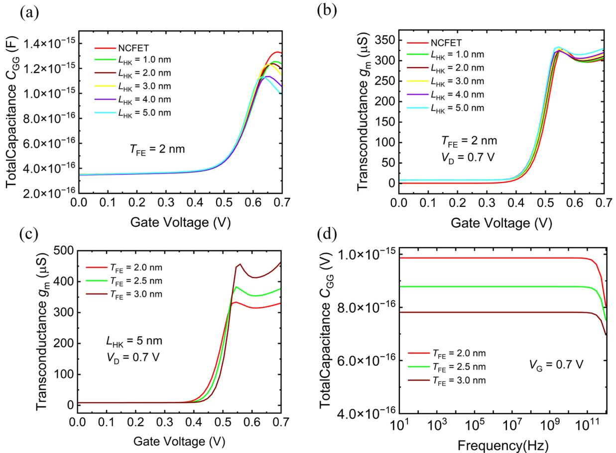
**Figure 7:** (a) total capacitance ( $C_{GG}$ ) curves as a function of the gate voltage at different  $L_{HK}$  values. (b) transconductance ( $g_m$ ) curves as a function of the gate voltage at different  $L_{HK}$  values. (c)  $g_m$  curves as a function of the gate voltage at different  $T_{FE}$  values. (d)  $C_{GG}$  curves as a function of the frequency at different  $T_{FE}$  values.
