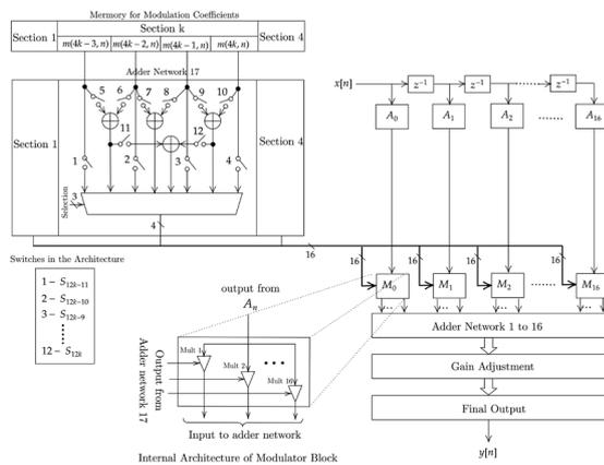
**Figure 6:** Architecture of the Proposed Non-Uniform Reconfigurable CMFB
