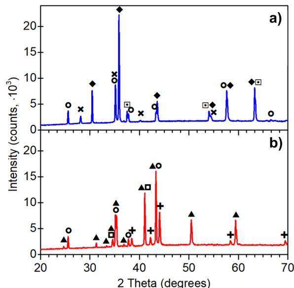
**Figure 2:** XRD patterns of a) 2113-30/air, and b) 2113-30/Ar. ◆: Ni-Mn-Co-O, ▲: alloys, ✕: RuO<sub>2</sub>, +: Ru, ○: Al<sub>2</sub>O<sub>3</sub>, □: cubic SiO<sub>2</sub> and ◻: orthorhombic SiO<sub>2</sub>.
