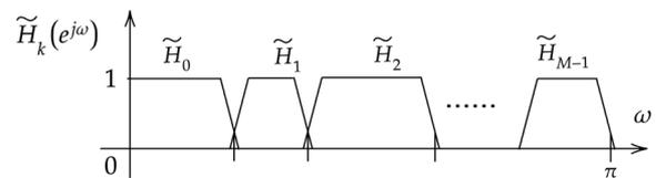
**Figure 5:** Magnitude Response of  $M$  Channel Non-uniform CMFB
