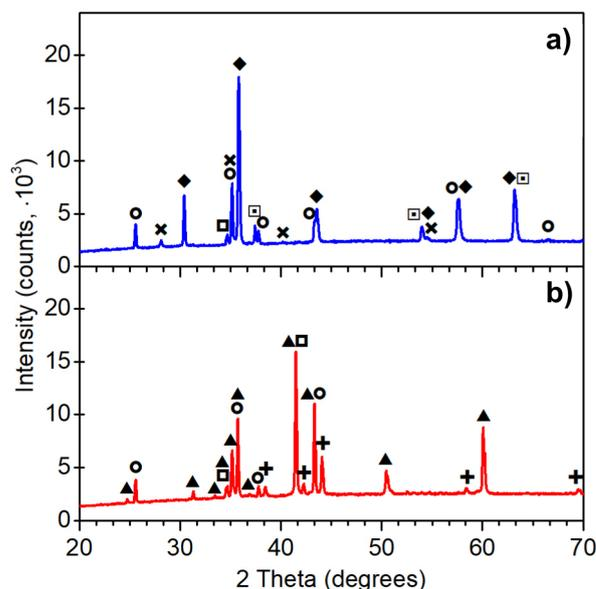
**Figure 3:** XRD patterns of a) 2114-30/air, and b) 2114-30/Ar. ◆: Ni-Mn-Co-O, ▲: alloys, ✕: RuO<sub>2</sub>, +: Ru, ○: Al<sub>2</sub>O<sub>3</sub>, □: cubic SiO<sub>2</sub> and ◻: orthorhombic SiO<sub>2</sub>.
