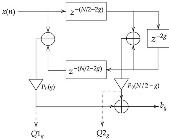
**Figure 8:** Implementation of the Sub filter component  $A_g$
