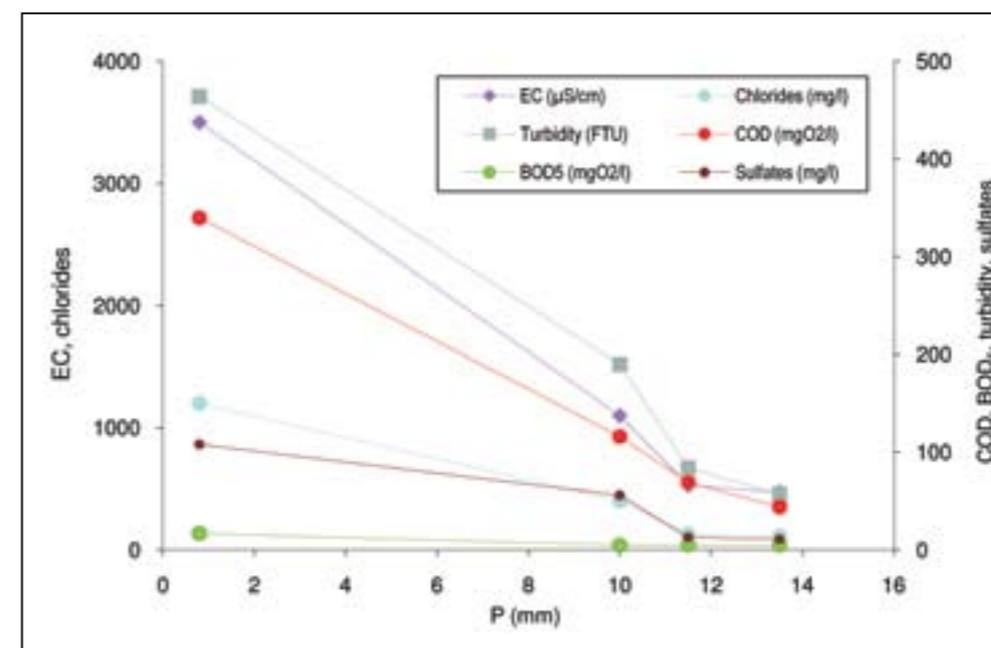
Fig. 2: Progress of measured parameters of oil collector inflow (EC, COD and BOD<sub>5</sub>) following a precipitation event on 24 March 1993 depending on the quantity of precipitation.
