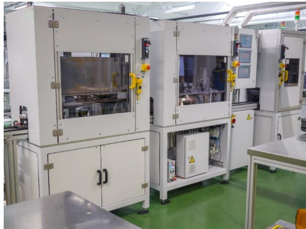
**Fig. 2** Modular EoL quality inspection system
