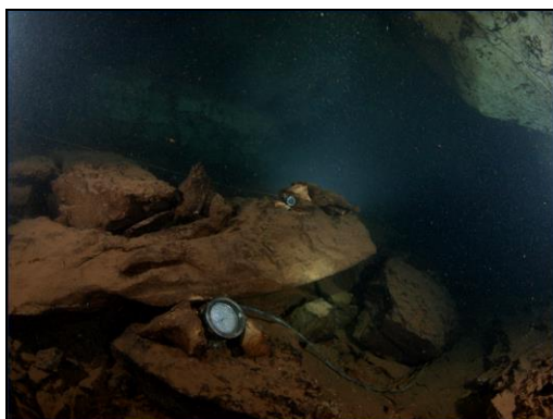
Figure 2. Installation of an IR camera with integral IR lights (top) and an independent stand-alone IR LED emitter array below it (photo: A. Sári).
