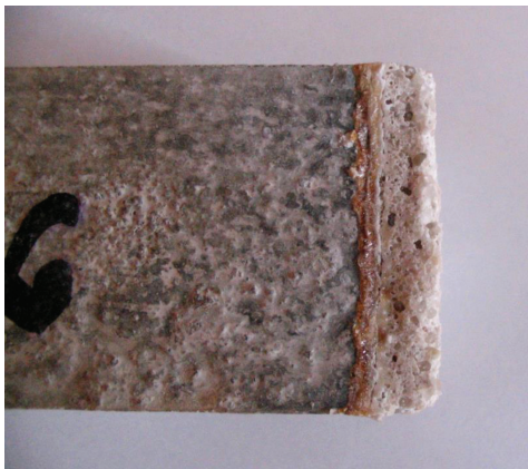
Figure 1: Lower part of SRP concrete sample after being in \text{H}_2\text{SO}_4 0.5 % for 6 months
