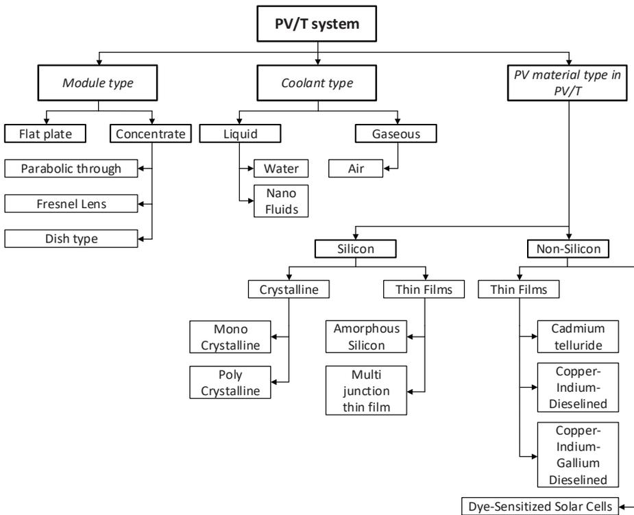
Figure 2: Schematic division of PV/T modules (redrawn from [3]).
