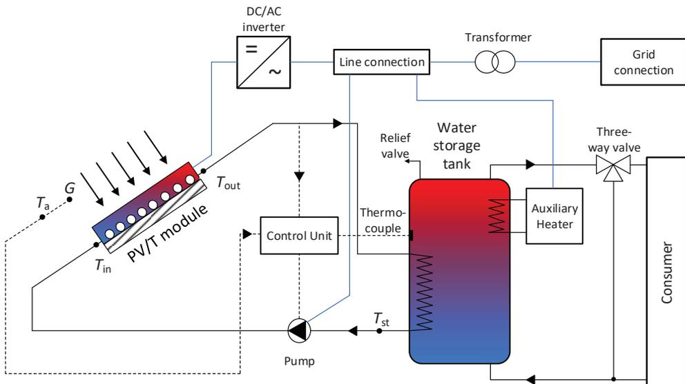
**Figure 1:** A simplified scheme of PV/T system.
