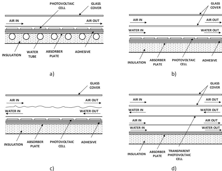
**Figure 3:** Schematics of the various PV-T air/water modules (redrawn from [1]): a) airflow before PV module and water flow in the tube (commercial type of water cooling), b) air/water flow (separated) before PV module, c) air/water flow (combined) before PV module and d) air/water flow (separated) before PV module and air/water flow (combined) behind PV module.
