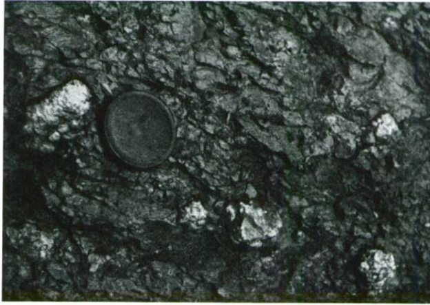
Sl. 7. Lapor z apnenimi in dolomitnimi gomolji Fig. 7. Marl including calcareous and dolomitic nodules
