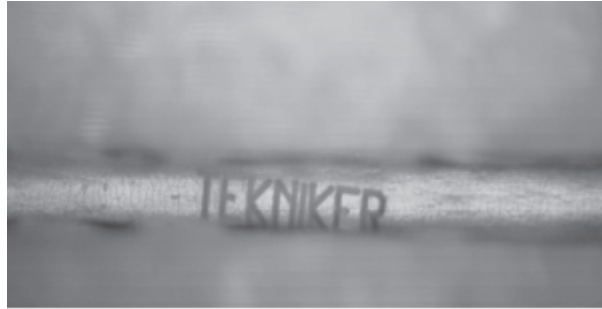
Fig. 1. A hair machined by a femto-second laser (image captured by x20 confocal microscope)
