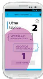
Figure 3: Thumb zones on the phone screen (right-handed user)
