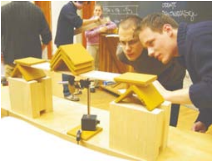
Slika 1: Upogibni preizkus na posameznem preizkušancu iz lesa v predavalnici Fakultete za arhitekturo (Foto: Edo Wallner). Bending test on a particular wooden sample carried out in the lecture hall at the Faculty of architecture.
