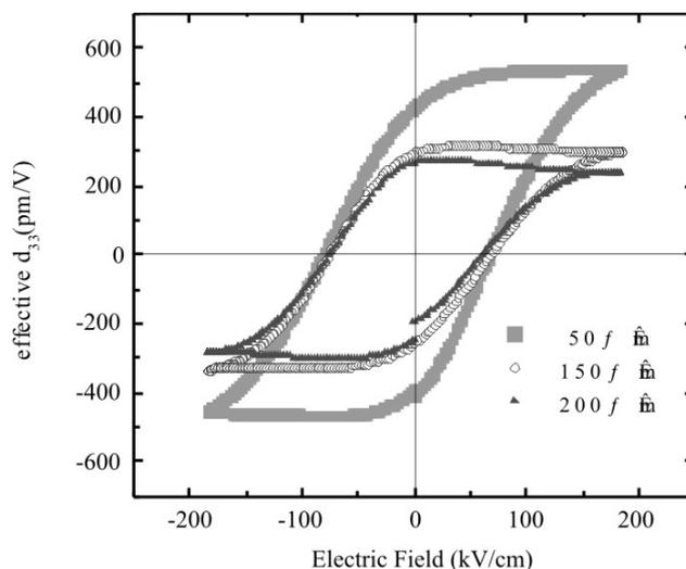
Fig.9 Effective  $d_{33}$  for PZT thin films with a MPB composition and different residual thickness of Si substrate.
