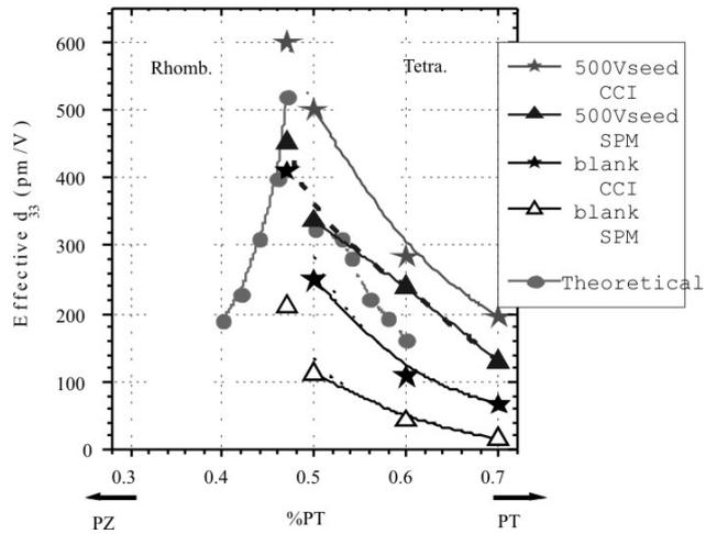
Fig.7 Relation between effective  $d_{33}$  and composition of PZT thin films with different orientations.
