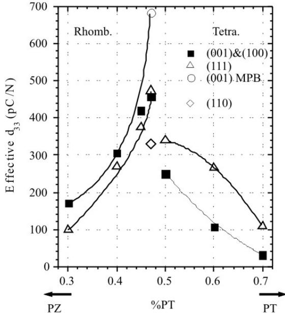
Fig.5 Relation between effective  $d_{33}$  and the compositions for PZT thin films with different film orientations.
