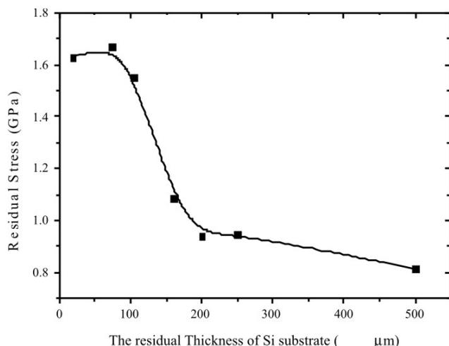
Fig. 8 Relation between residual stress in films and residual thickness of Si substrate measured by raman spectroscopy<sup>13)</sup>.
