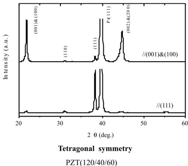
Fig.3 a XRD patterns for PZT thin films with tetragonal symmetry.
