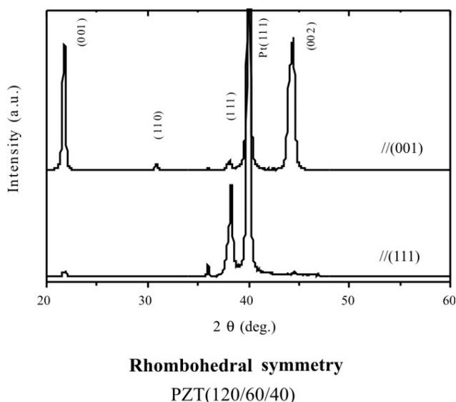
Fig.3 b XRD patterns for PZT thin films with rhombohedral symmetry.
