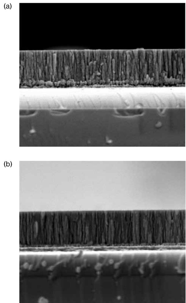
Fig.4 Cross-sectional SEM images for CSD-derived PZT thin films of MPB composition with (a) (111)- and (b) (001)&(100)- orientation.
