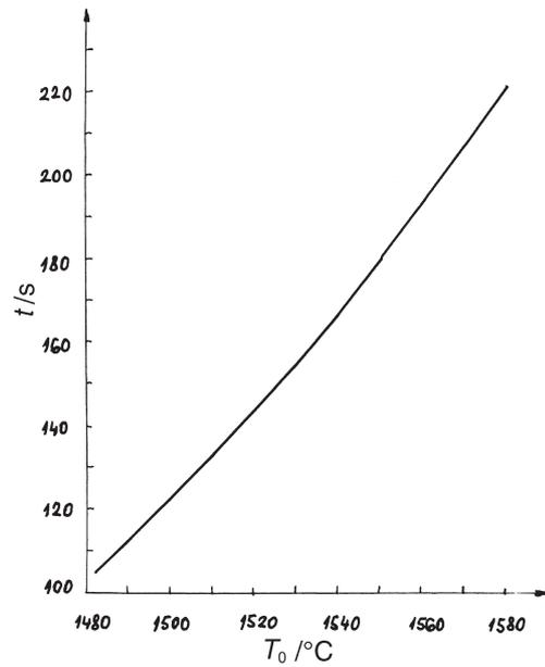
**Figure 5:** Dependence cooling time for the surface temperature of 1000 °C versus strand initial temperature for a casting machine with standard cooling
