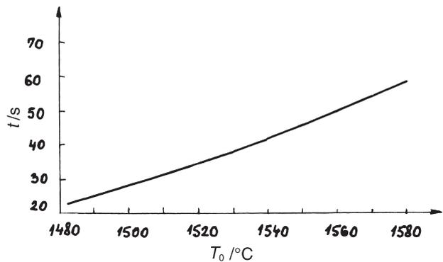
Figure 2: Dependence cooling time for the surface temperature of 1164 °C versus strand initial temperature in zone II
