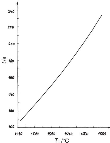
**Figure 4:** Dependence cooling time for the surface temperature of 1036 °C versus strand initial temperature in zone IV
