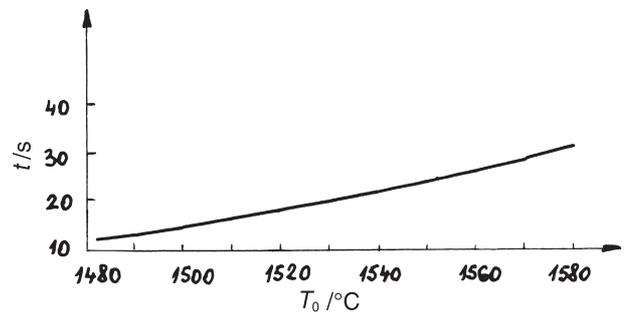
Figure 1: Dependence cooling time for the surface temperature of 1193 °C versus strand initial temperature in zone I
