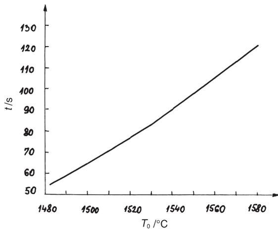
**Figure 3:** Dependence cooling time for the surface temperature of 1064 °C versus strand initial temperature in zone III
