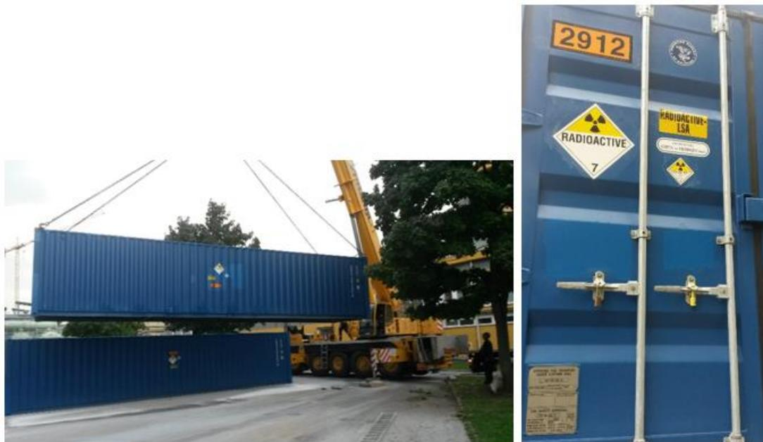
**Figure 18: Manipulations of the ISO container with a crane at Cinkarna Celje, d.d. (left); markings on the ISO container and seal (right) (Photo: SNSA inspection service)**
