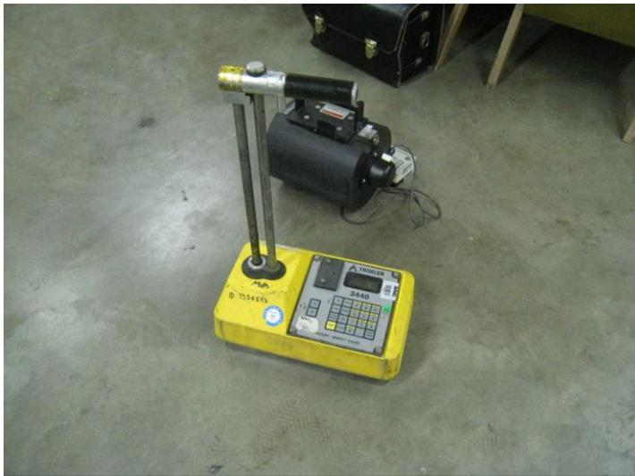
**Figure 14: TROXLER 3440 gauge with defective movement mechanism (Photo: IOS)**
