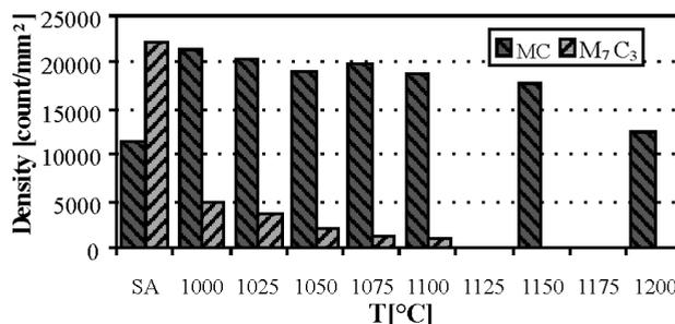
**Figure 4:** The density of carbides as a function of the austenitizing temperature
