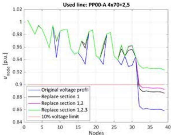
**Figure 17:** Voltage profile with conductor type PP00-A 4x70+2.5 in selected sectors
