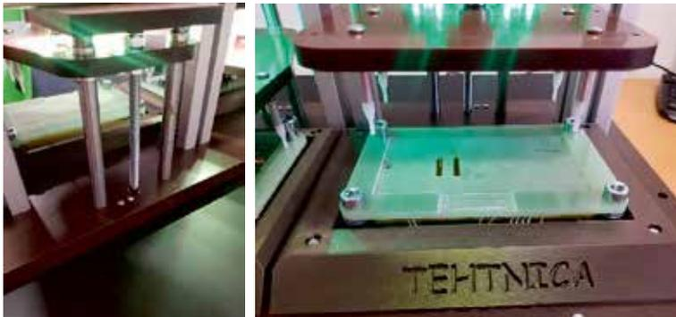
**Figure 4:** Clamping mechanism
