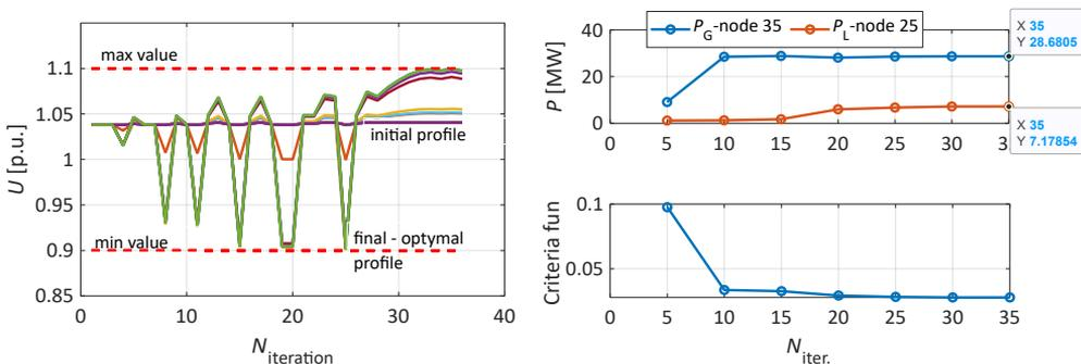
**Figure 15:** Voltage profile in all thirty-five nodes while adding a generation unit into node 35 (left) and adding load to node 25, optimisation evolution on the right
