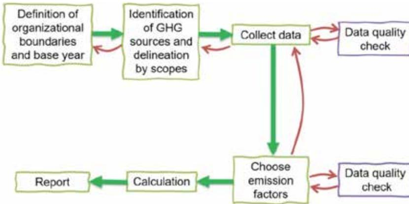
*Figure 3: Workflow of the carbon footprint methodology*
