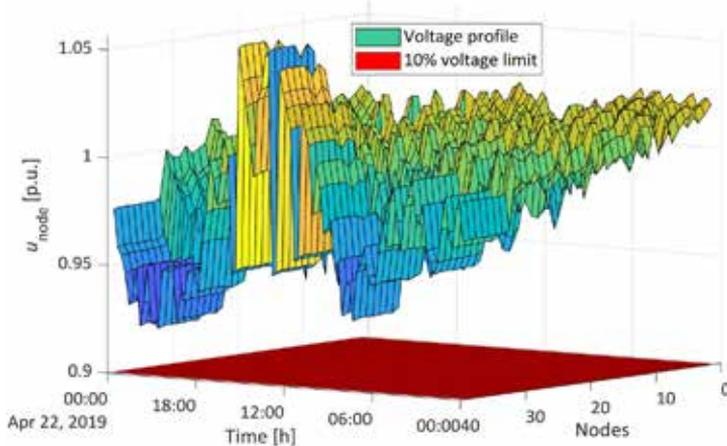
**Figure 14:** Voltage profile over time and nodes with PV power plant and BESS at node 35
