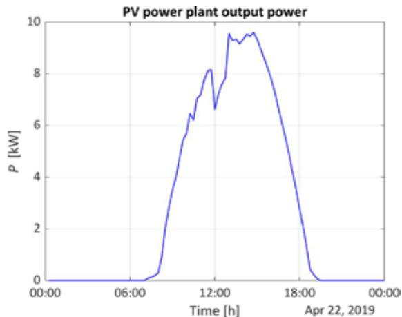
Figure 11: Output power profile of PV power plant over time
