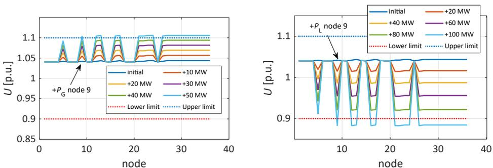
Figure 8: Voltage profile in all thirty-five nodes while adding generation unit into node 9 (left) and adding load (right)
