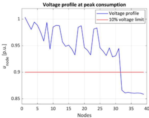
Figure 6: Voltage profile over nodes for the moment of highest consumption
