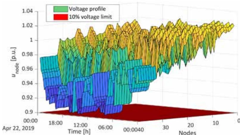
Figure 10: Voltage profile over time and nodes with BESS at node 27
