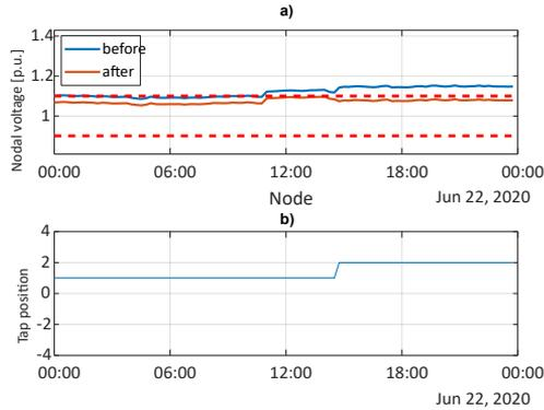
**Figure 13:** Voltage before and after the application of the OLTC and display of the degree of OLTC taps for the selected case over time
