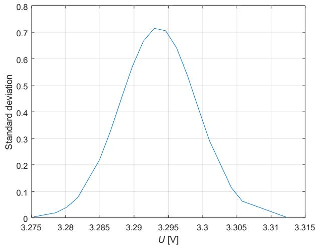
**Figure 9:** Normal distribution of the 3.3 V linear regulator
