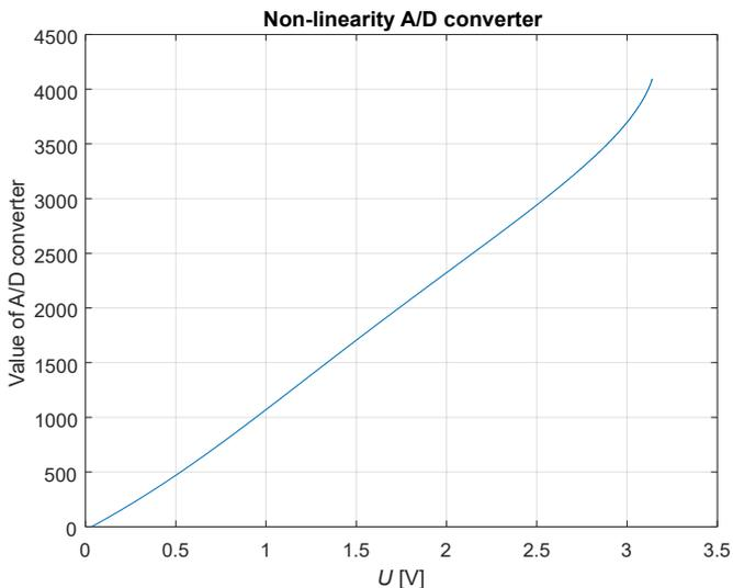
**Figure 6:** Non-linearity of the ADC
