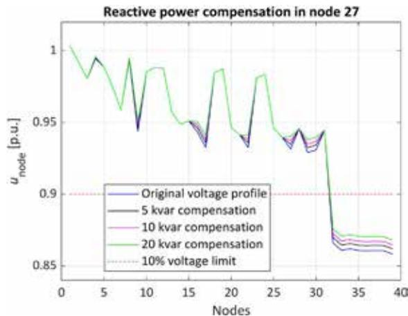
Figure 8: Voltage profile with reactive power compensation device
