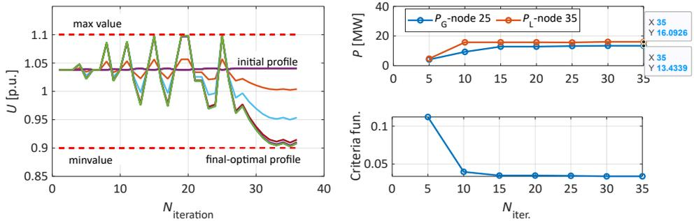
**Figure 16:** Voltage profile in all thirty-five nodes while adding a generation unit into node 28 (left) and adding load (right)
