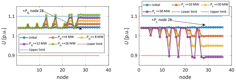
**Figure 9:** Voltage profile in all thirty-five nodes while adding generation unit into node 28 (left) and adding load (right)
