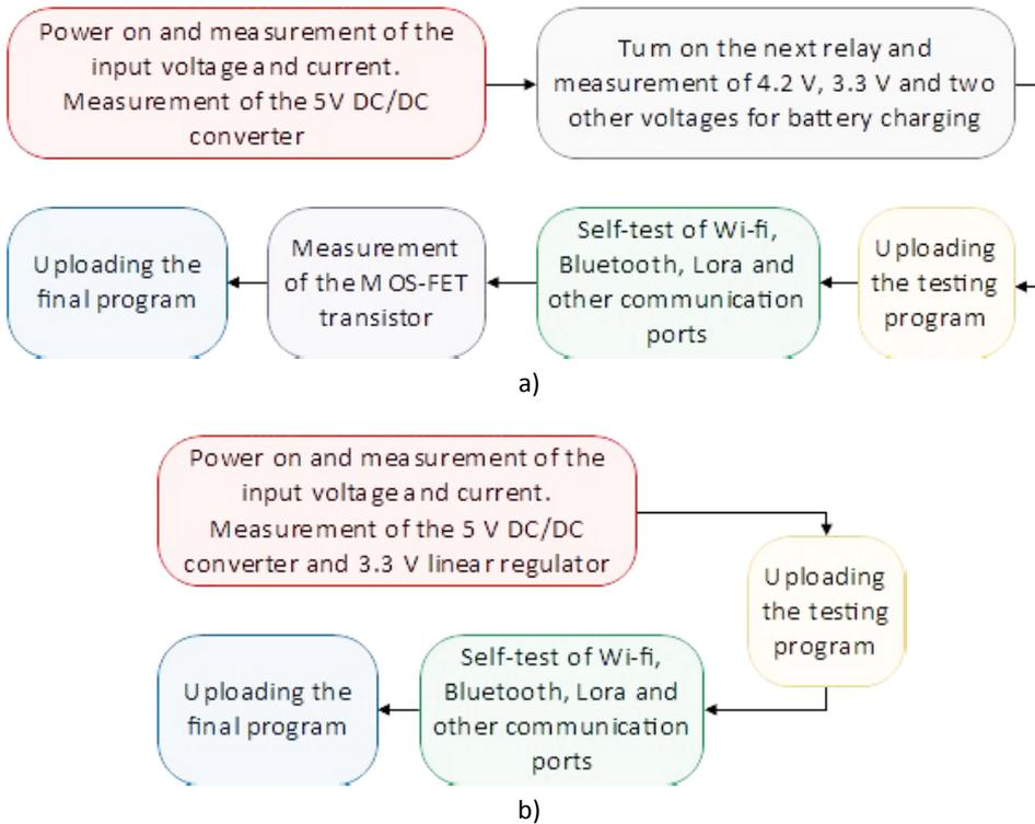
**Figure 2:** Protocol of measurements for the first (a) and second (b) PCBA
