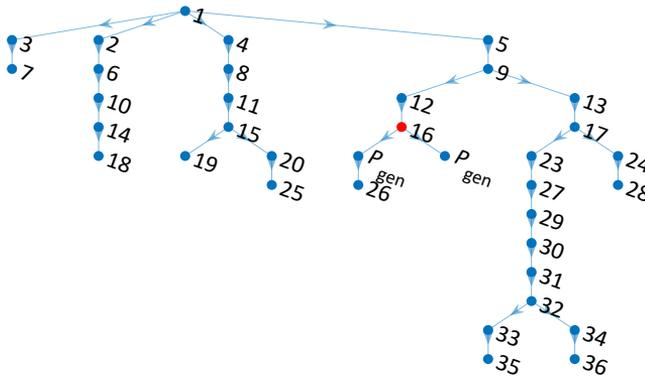
**Figure 11:** Topology of considered radial distribution network with marked node with OLTC and nodes of additional generation units
