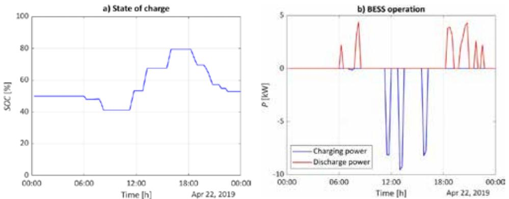
**Figure 13:** SOC (a) and operation of BESS (b) at node 35 over time in combination with PV power plant
