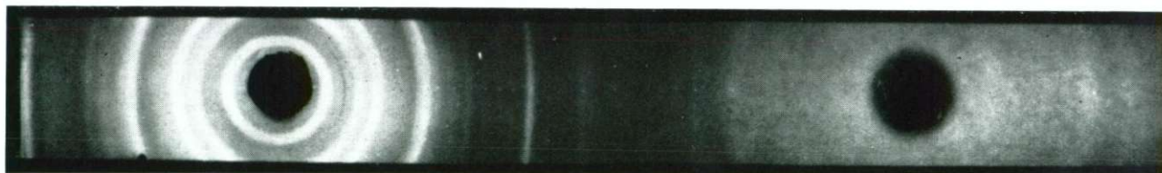
2. sl. Debeygram korlačanskega azbesta z jalovino (kobaltova anoda) Fig. 2. X-rays diffraction pattern of the Korlača-asbestos with the waste (Co anticathode)
