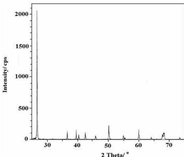
Figure 1. XRD spectrum of untreated tripoli.
