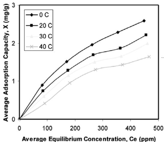
Figure 3. Average adsorption capacity of cadmium ion against average equilibrium concentration, at 0, 20, 30 and 40 °C.
