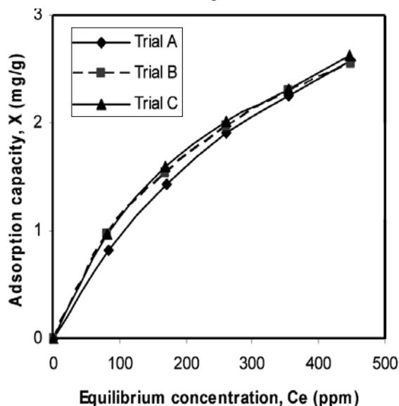
Figure 4. Adsorption capacity of cadmium ion against equilibrium concentration, at 0 °C for the trials A, B and C.
