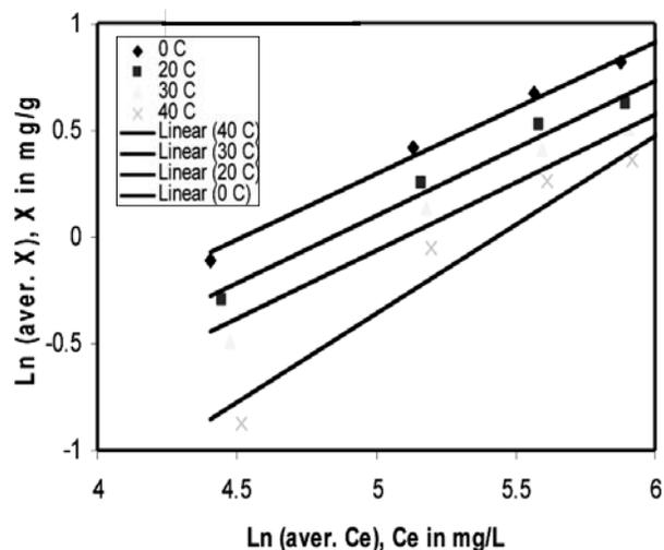
**Figure 5.** Freundlich lines,  $\ln(\text{average } X)$  against  $\ln(\text{average } C_e)$ , for the adsorption of Cd(II) at 0, 20, 30 and 40 °C.
