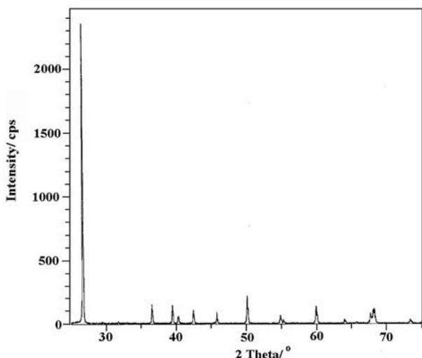
Figure 2. XRD spectrum of untreated tripoli.
