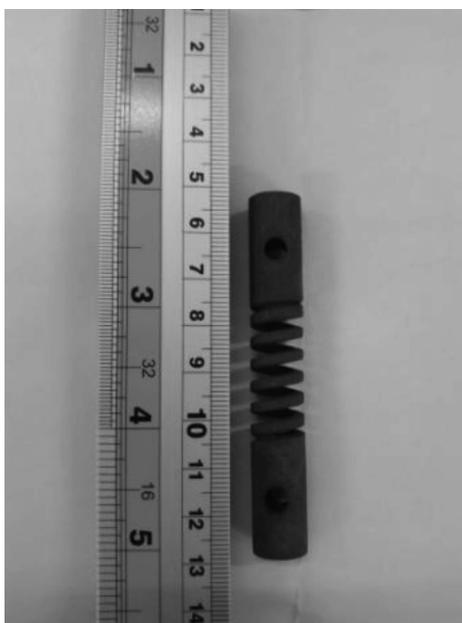
**Figure 1:** Helicoidal-spring specimen for the stress-change testing
