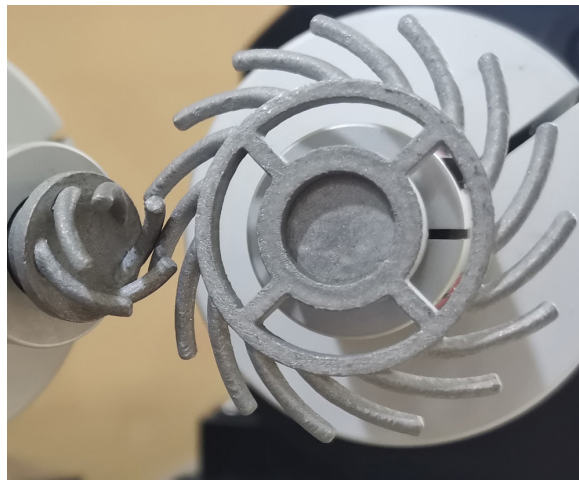
Fig. 1. Space curved cantilever beams on a pair of line gears
