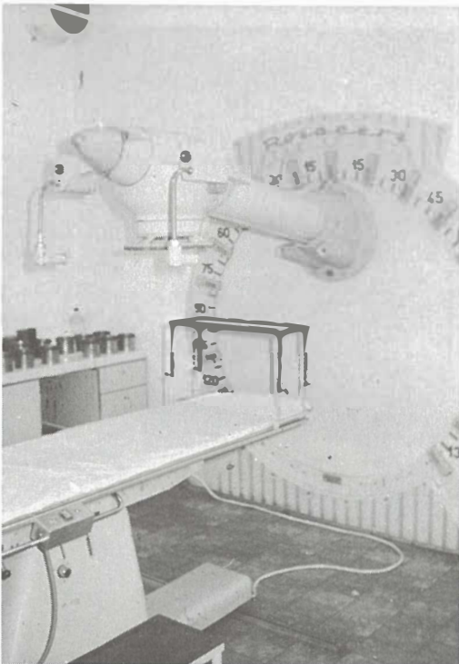
Figure 2. The Rotacert, made by Medicor Co., working with gravicert principle.
