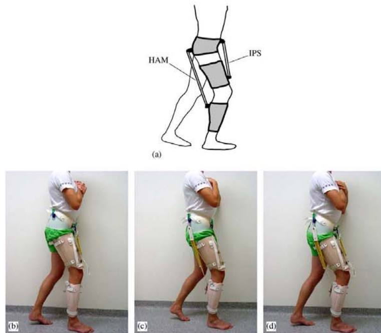
Fig. 1. a. Schematic presentation of a walking subject, wearing pelvic, thigh and shank cuffs upon which two artificial muscles, one emulating iliopsoas (IPS) muscle contracture and the other hamstrings (HAM) muscle contracture, are attached. b. IPS applied. c. HAM applied. d. IPS and HAM applied.
