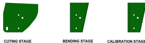
Figure 1. Conventional sheet metal forming tool strip layout example
