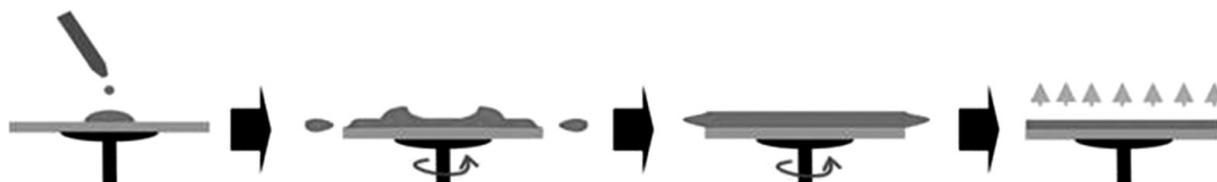
**Figure 1:** Scheme of the spin-coating sensor preparation
