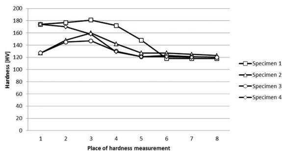
Figure 6: Course of hardness on the welded specimens.
