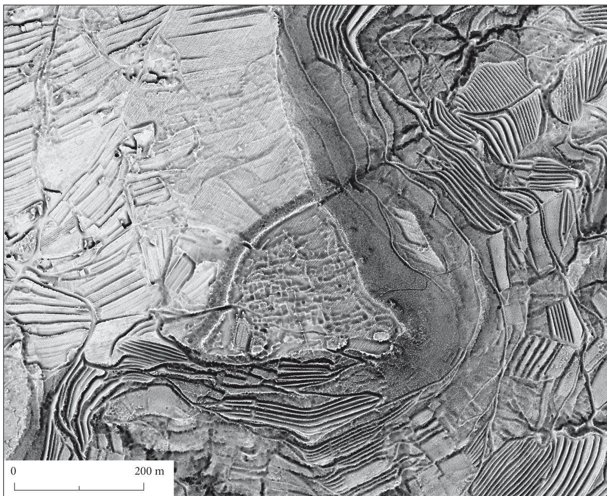
Fig 2: Sv. Pavel above Planina, 0.5 m lidar derived digital elevation model revealing Roman-period building features.
