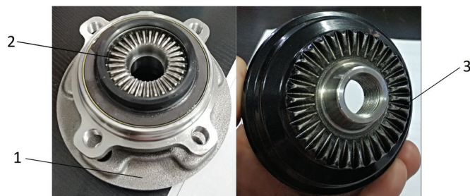
Fig. 6. Generation III wheel hub unit with a torque transmission gear system; 1 outer flanged ring, 2 inner flanged ring with a face gear and 3 halfshaft gear with meshing teeth
