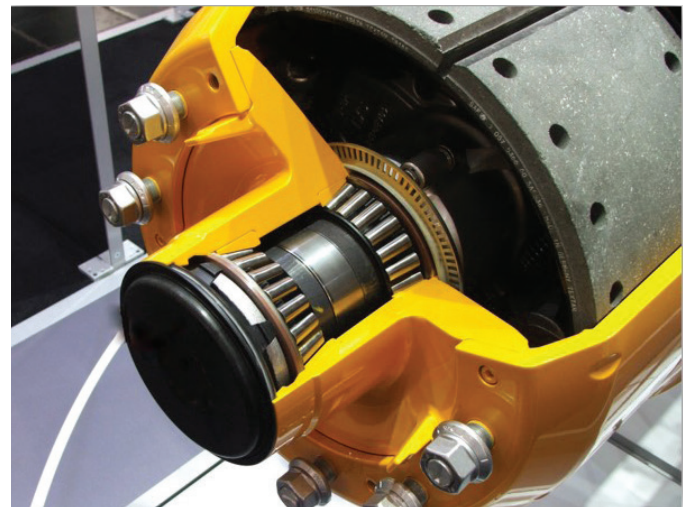
Fig. 1. Wheel hub unit with two tapered roller bearings
