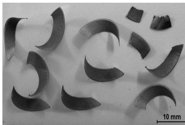
Figure 8: Chip formation at V = 90 m/min
