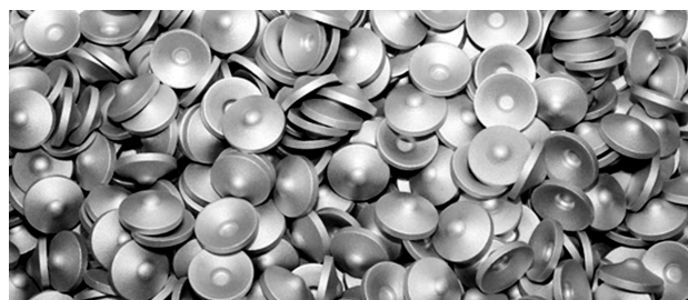
Figure 3: Slugs produced in the Talum Al factory used as semi-products in the production of tubes and containers in the pharmaceutical, food and cosmetic industries 8
