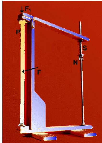
**Figure 1.** A harmonic oscillator realised with a steel strip **P** fixed at its ends. When a force **F** is applied perpendicular to the strip, the system tends to return to its equilibrium position. The spring **S** can apply a force  $F_1$  regulated by the nut **N**.
