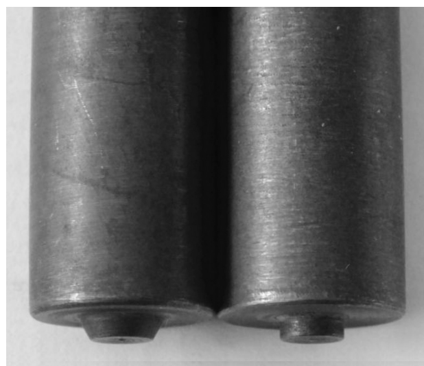
Figure 2: Two types of tool used for FSSW: FSSW-T (tapered pin, left) and FSSW-C (circular pin, right)
