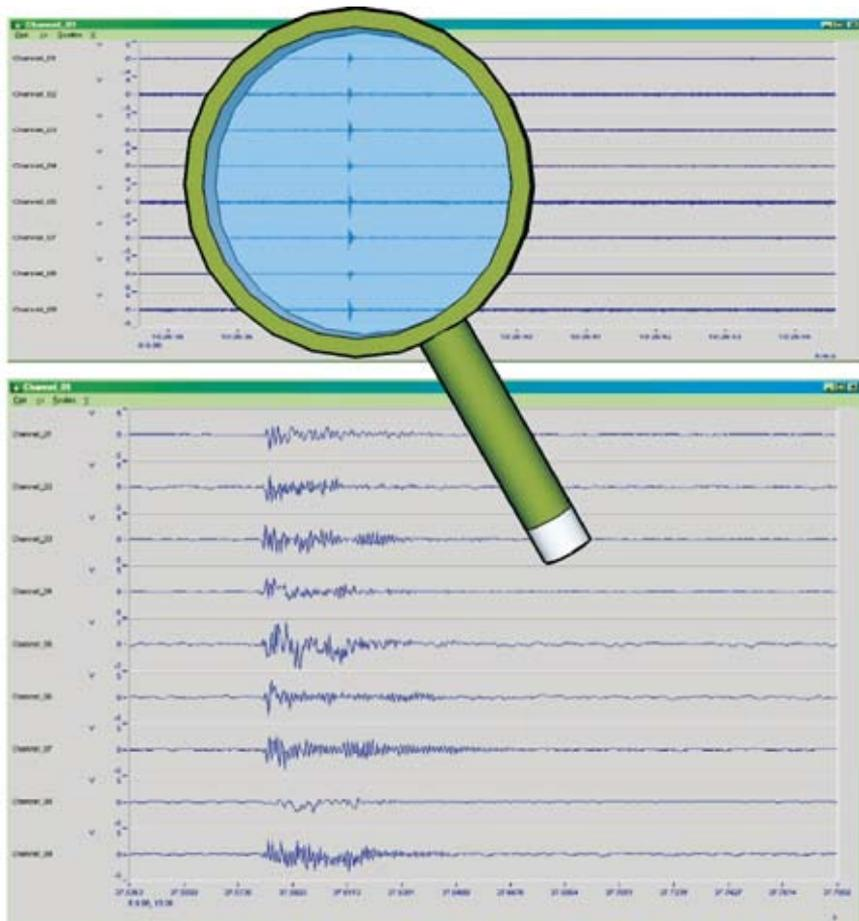
**Figure 4.** An example of the accelerogram recorded by the in-mine system. Time is in seconds, amplitude in Volts.
