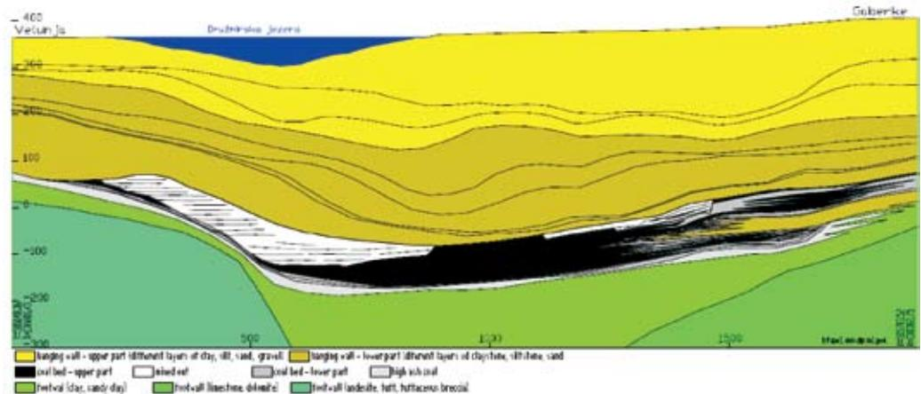
**Figure 1.** Longitudinal section of the coal seam (geomechanical interpretation)
