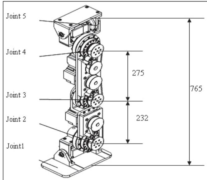
**Figure 3.** The schematic structure of a mechatronic lower limb
