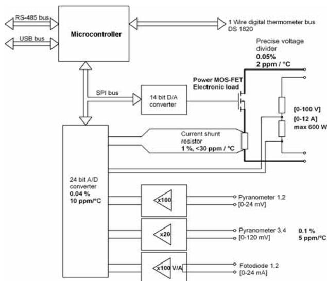
Fig. 4: Block diagram of the PV measurement unit.
