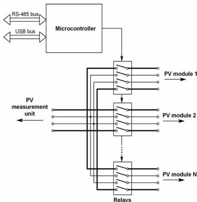
Fig. 5: Block diagram of the 4-point module switching unit.
