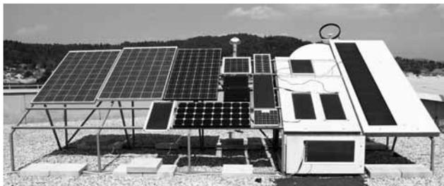
**Fig. 2:** Outdoor PV module monitoring site located on the roof of the Faculty of Electrical Engineering in Ljubljana.
