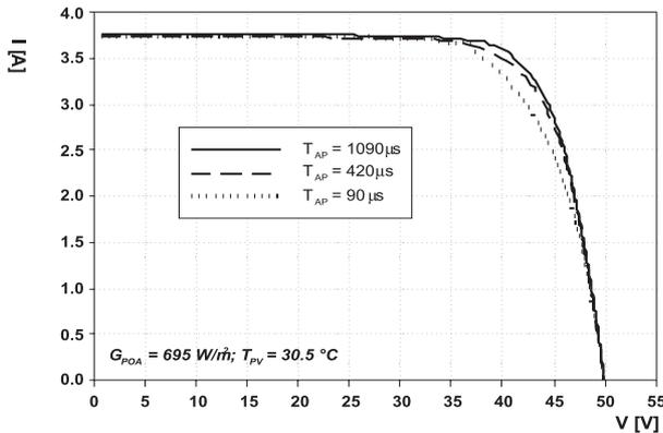
Fig. 7: Measured I-V curves of the Sanyo HIT PV module at different  $t_{AP}$  ( $t_{AP} = 1090 \mu s$  – solid line,  $t_{AP} = 420 \mu s$  – dashed line and  $t_{AP} = 90 \mu s$  – dotted line).
