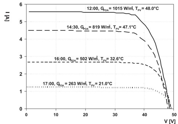
Fig. 9: Measured I-V curves of a Sanyo HIT PV module on the 30<sup>th</sup> of March 2008.
