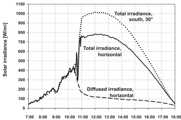
**Fig. 10:** Total (solid line) and diffused solar irradiance (dashed line) on flat surface and total solar irradiance on plane of array (dotted line) on the 30<sup>th</sup> of March 2008.
