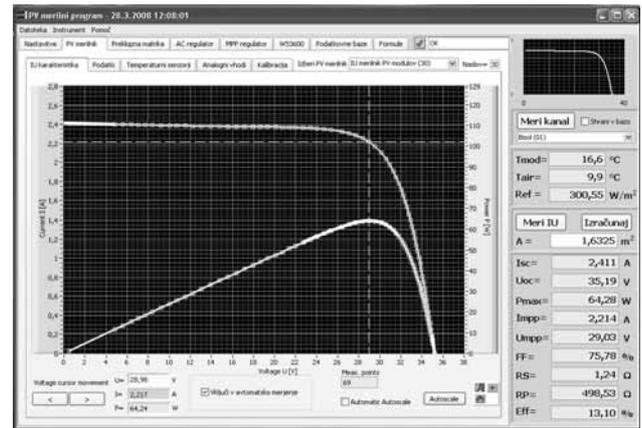
Fig. 8: Screen shot of the measurement software developed in program language LabVIEW.
