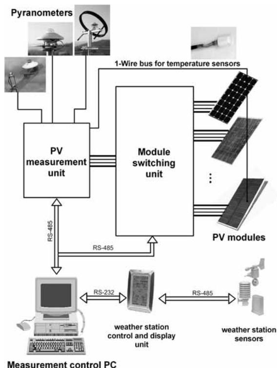
Fig. 3: Block diagram of the PV monitoring system.
