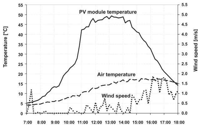
**Fig. 11:** HIT PV module temperature (solid line), air temperature (dashed line) and wind speed (dotted line) on the 30<sup>th</sup> of March 2008.
