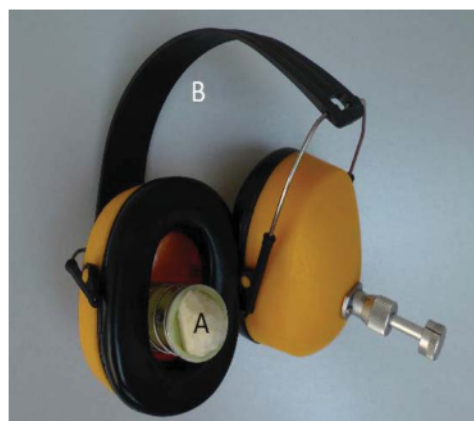
Figure 3: Dummy earphones: A – latex sponge pads mounted on the soft springs for arrest of plugs in outer ear, B – dummy headphones
