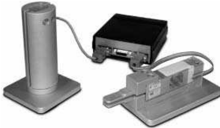
Fig. 1. A compact assessment system with two force measuring units in the shape of a cup and thin plate can be connected to a personal computer to accurately measure the dynamic grip force in cylindrical and lateral grip.
