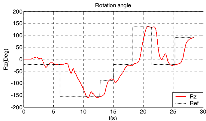
Figure 6.13: Rotation angle of the knob during the safe opening. The dotted reference line represents the required orientation for the code "AGDA6A4".
