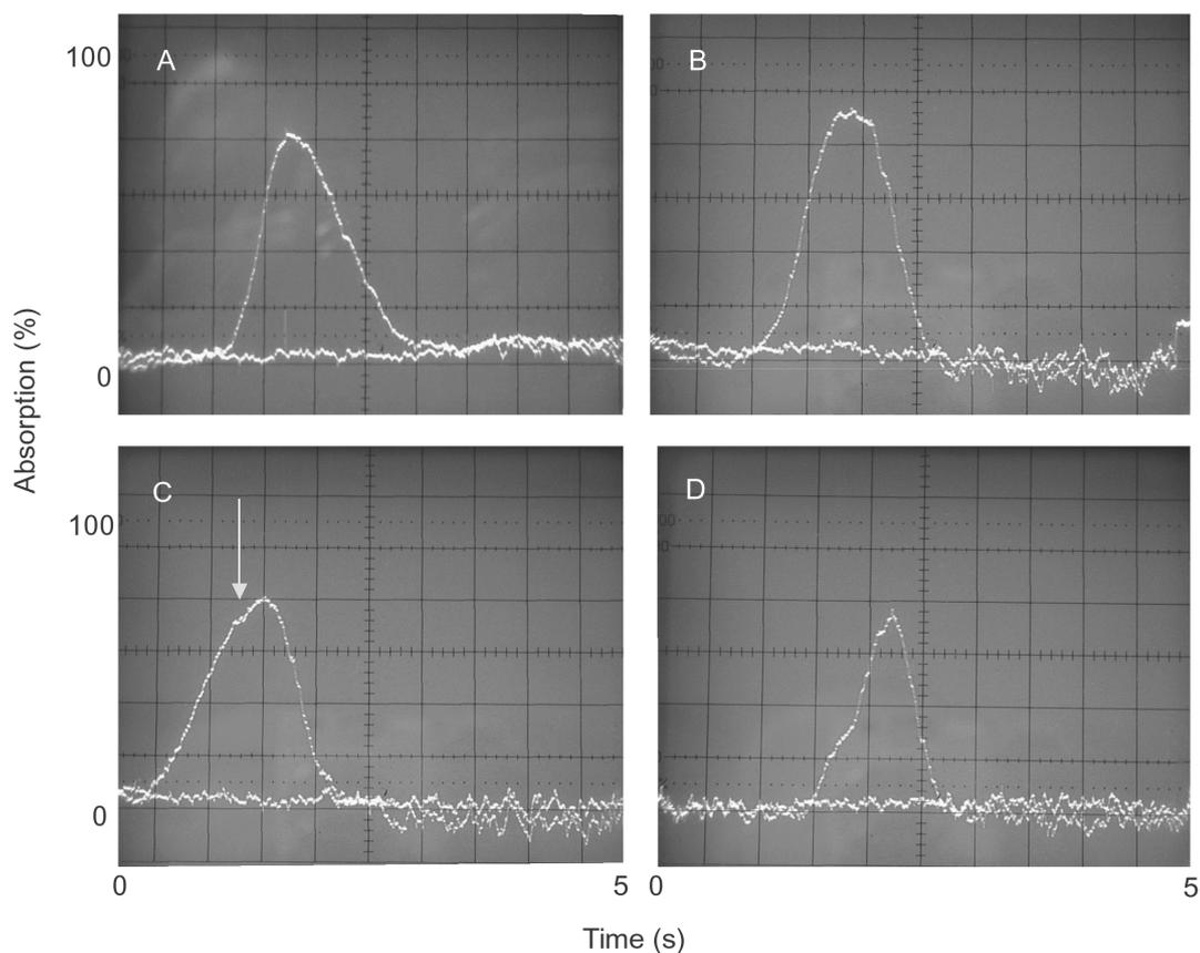
**Figure 5.** Absorption-time profiles of cadmium resulting from atomization of aqueous standard and various biological solid samples employing the direct »tape sandwich« introduction technique; A – CdCl<sub>2</sub>; B – powdered hair; C – cabbage; D – bovine liver.
