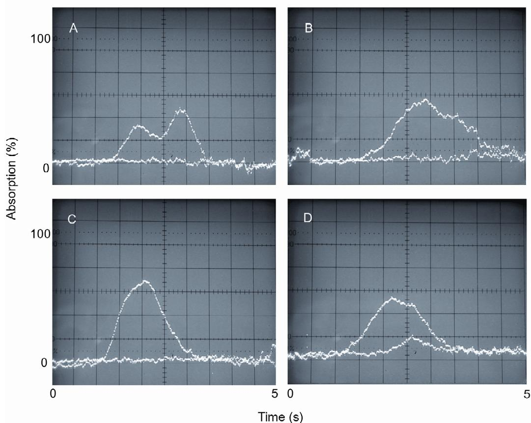
**Figure 4.** Absorption-time profiles of lead resulting from atomization of different plant materials employing the direct »tape sandwich« and slurry introduction techniques; A – lettuce – direct introduction: B – Sea Lettuce – direct introduction: C – lettuce – slurry introduction: D – Sea Lettuce – slurry introduction.
