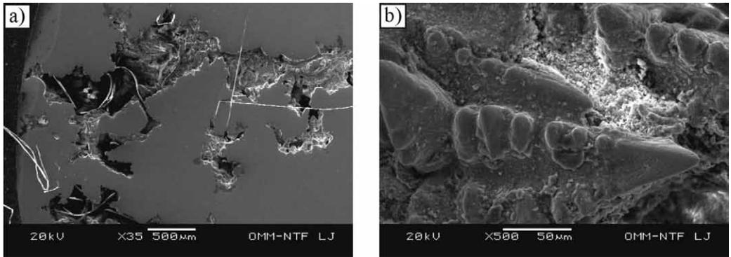
**Figure 9.** Microstructures of the steel product in the central zone obtained using SEM at different magnifications, 1st position.
