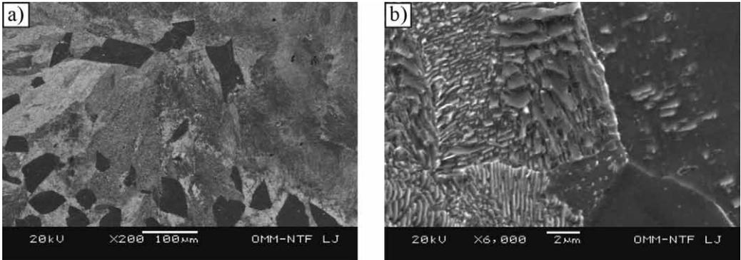
**Figure 4.** Microstructures of the steel product in the central zone obtained using SEM at the different magnification.
