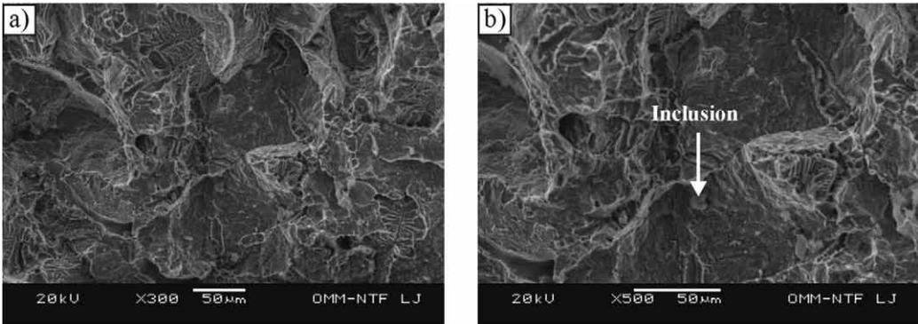
**Figure 11.** SEM micrographs of fracture surface near the surface of the round cross-section at different magnifications.
