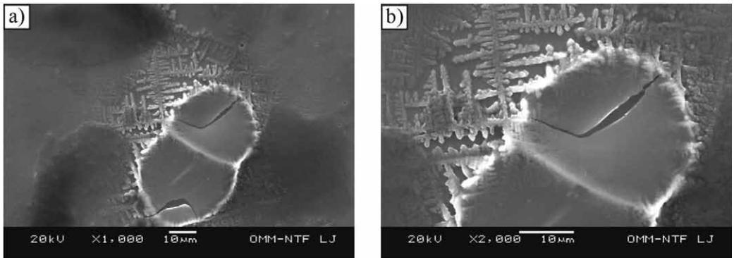
**Figure 10.** Microstructures of the steel product in the central zone obtained using SEM at different magnifications, 2nd position.
