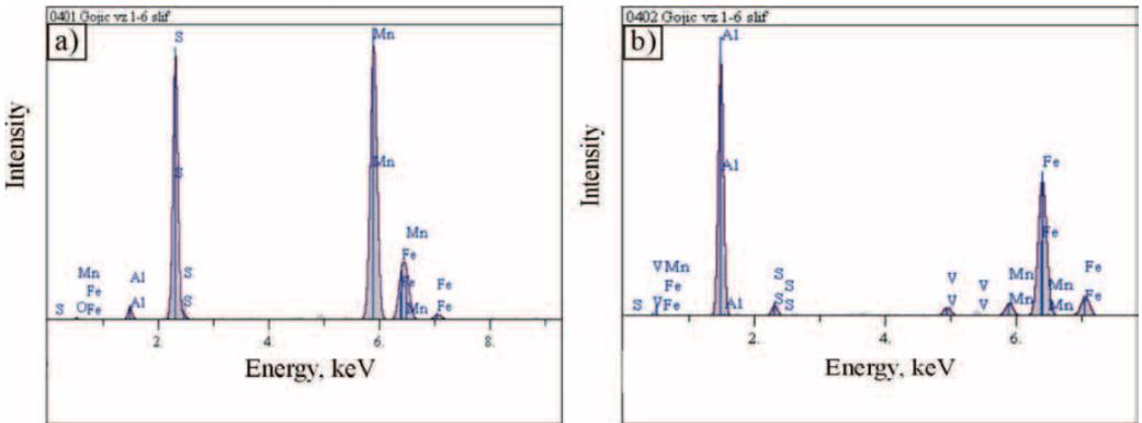
**Figure 8.** EDX spectra of particles enriched with sulphur (a) and aluminium (b) at the ferrite/pearlite interface shown in Figure 7a.
