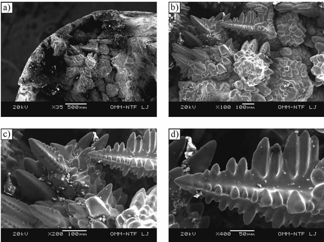
**Figure 12.** SEM micrographs of fracture surfaces in the central zone of the round cross-section at different magnifications.
