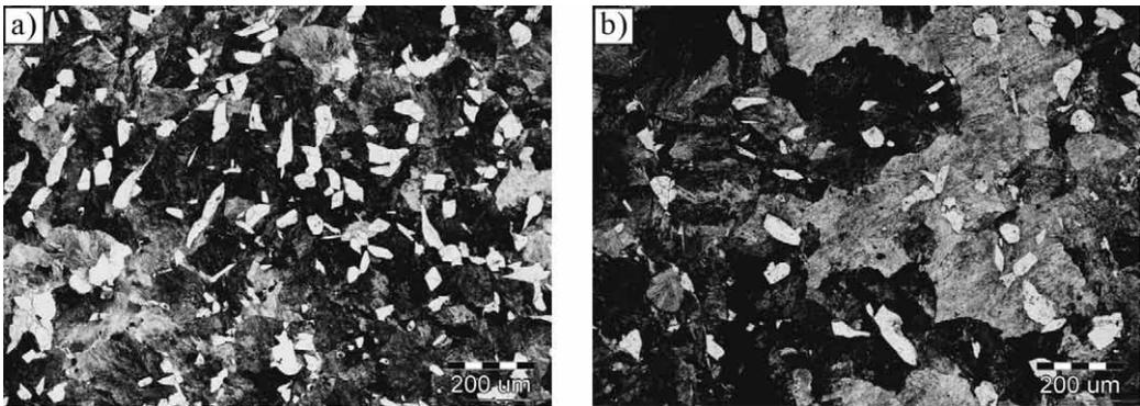
**Figure 2.** Microstructures of the steel product near the outer surface (a) and in the central zone (b) obtained using OM on specimens etched by nital solution.
