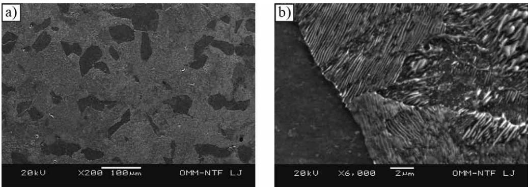
**Figure 3.** Microstructures of the steel product near the outer surface obtained using SEM at different magnifications.
