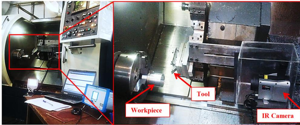
Fig. 2 The setup for measurement of the machining temperature in the CNC machine
