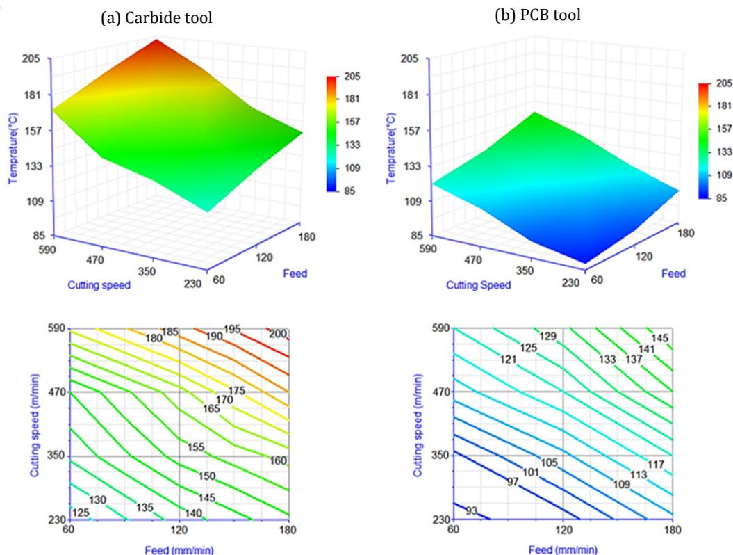
**Fig. 6** Experimental results of measured chip temperature for carbide tool (a) and PCD tool (b) versus feed rate and cutting speed changes
