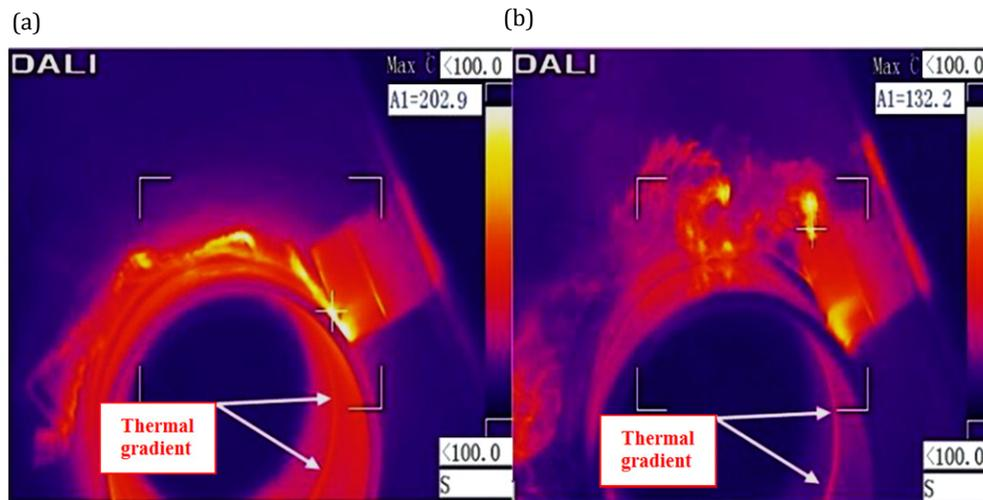
**Fig. 5** The transmission of the generated heat from cutting zone to the workpiece, and the creation of a thermal gradient in a section of the workpiece
