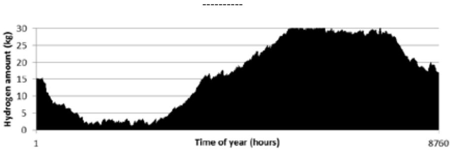
Figure 6: Hydrogen tank storage level during the year
