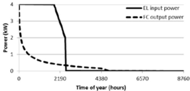
Figure 9: Electrolyser and fuel cell duration curves
