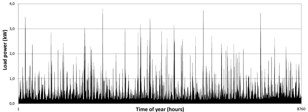
**Figure 2:** Hourly electricity consumption for a one-year period
