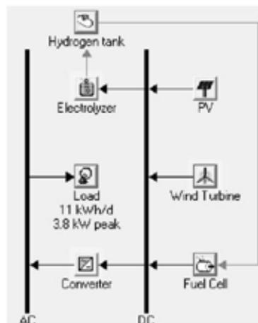
**Figure 1:** HOMER numerical model of a stand-alone energy system
