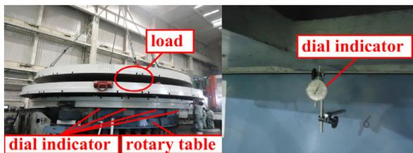
Fig. 11. Bearing capacity experiment setup
