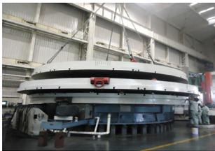
Fig. 9. The optimized hydrostatic rotary table
