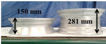
Fig. 7. Initial work piece and manufactured wheel
