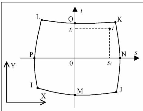
**Fig. 3.** Geometrical scheme of the finite element.
