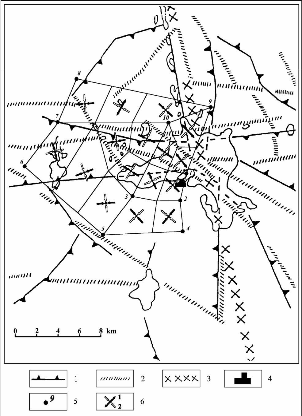
Fig. 4. Directions of changes of the principal geodynamic Earth-crust stresses (the finite element network consists of 16 quadrangles). Tectonic breaks (according to I. Juknelis, V. Marcinkevičius, I. Šeštokas and A. Šliaupa) discovered by: 1 – seismic survey, 2 – aeromagnetic survey, 3 – morphostructural analysis; 4 – Igalina nuclear power plant, 5 – GPS point, 6 – the principal stresses (1 – maximum change of the principal stress, 2 – minimum change of the principal stress).
