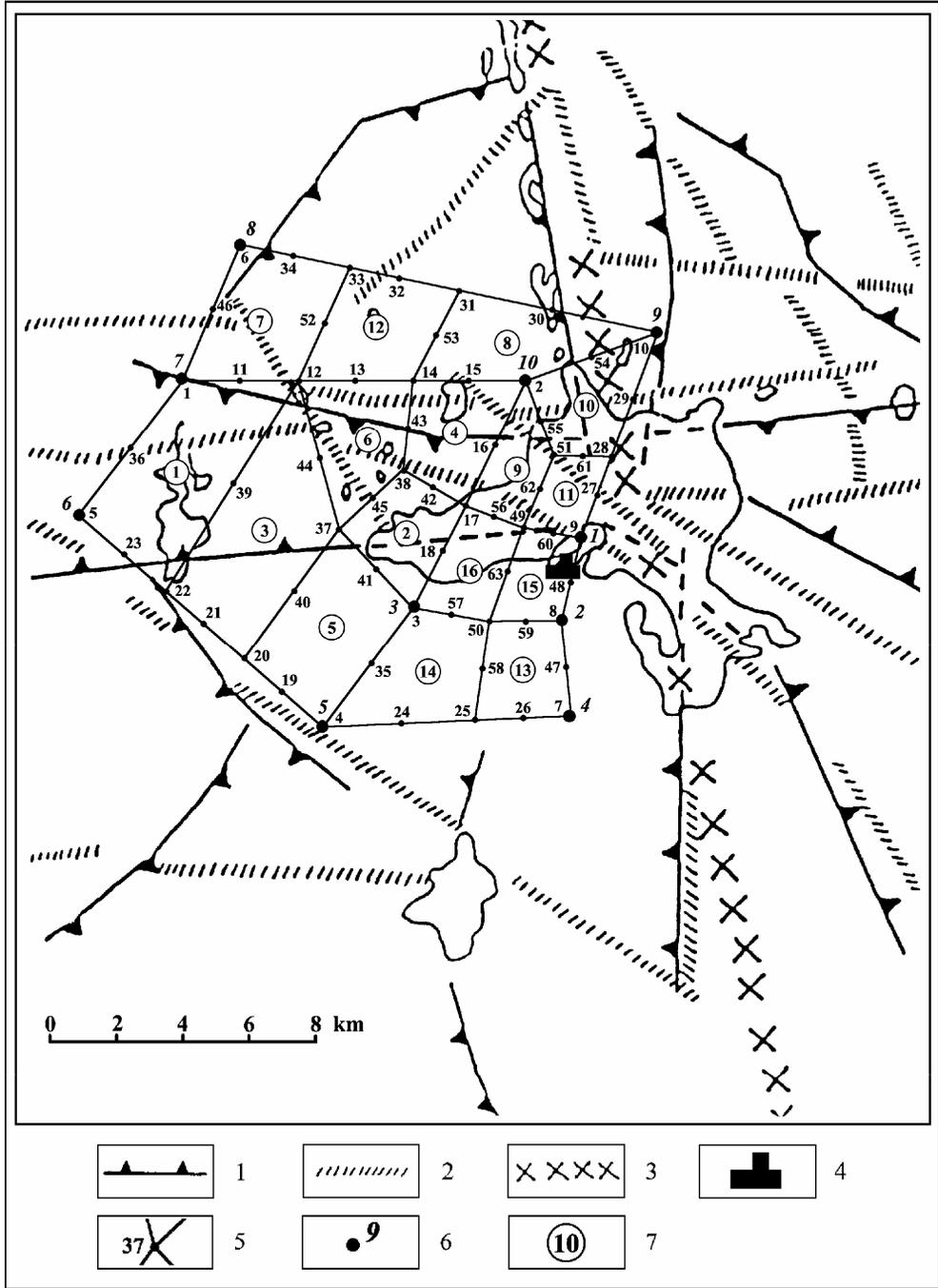
Fig. 1. The location scheme of the tectonic breaks and network of the finite elements at the Ignalina nuclear power plant (the finite element network consists of 16 quadrangles). Tectonic breaks (according to I. Juknelis, V. Marcinkevičius, I. Šeštokas and A. Šliaupa) discovered by: 1 - seismic survey, 2 - aeromagnetic survey, 3 - morphostructural analysis; 4 - Ignalina Nuclear Power Plant, 5 - finite element node, 6 - GPS point, 7 - finite element number.
