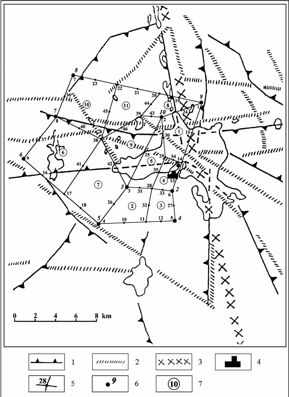
Fig. 2. The location scheme of the tectonic breaks and network of the finite elements at the Ignalina nuclear power plant (the finite element network consists of 11 quadrangles). Tectonic breaks (according to I. Juknelis, V. Marcinkevičius, I. Šeštokas and A. Šliaupa) discovered by: 1 – seismic survey, 2 – aeromagnetic survey, 3 – morphostructural analysis; 4 – Ignalina Nuclear Power Plant, 5 – finite element node, 6 – GPS point, 7 – finite element number.
