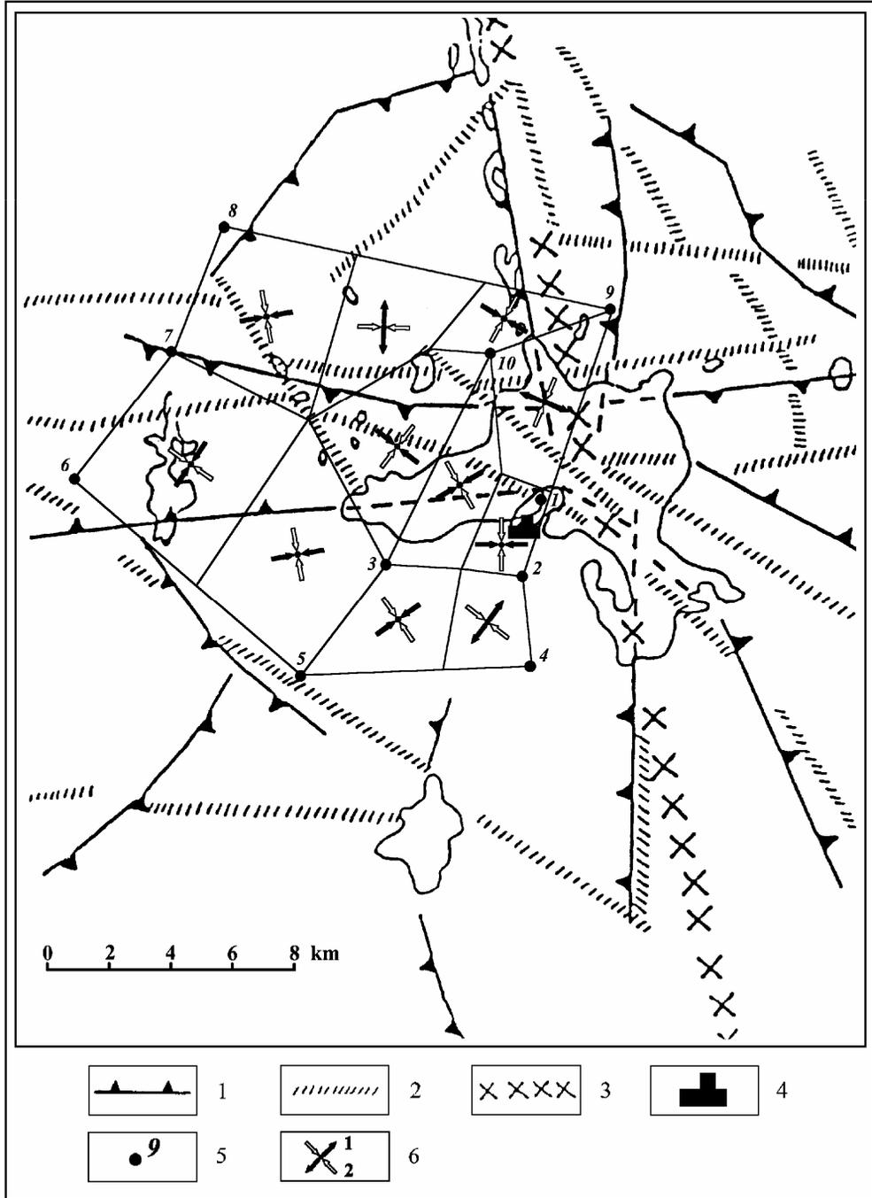
**Fig. 5.** Directions of changes of the principal geodynamic Earth-crust stresses (the finite element network consists of 11 quadrangles). Tectonic breaks (according to I. Juknelis, V. Marcinkevičius, I. Šeštokas and A. Šliaupa) discovered by: 1 – seismic survey, 2 – aeromagnetic survey, 3 – morphostructural analysis; 4 – Ignalina nuclear power plant, 5 – GPS point, 6 – the principal stresses (1 – maximum change of the principal stress, 2 – minimum change of the principal stress).
